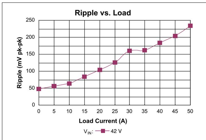
Figure 7 — V<sub>ripple</sub> vs. I<sub>OUT</sub>; No external C<sub>OUT</sub>. Board mounted module, scope setting: 20 MHz analog BW
