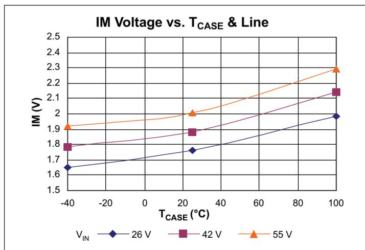
Figure 10 — Full load IM voltage vs. T<sub>CASE</sub>
