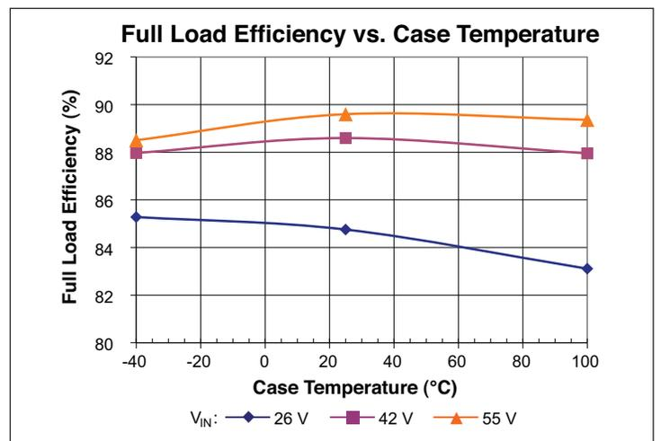
Figure 2 — Full load efficiency vs. temperature
