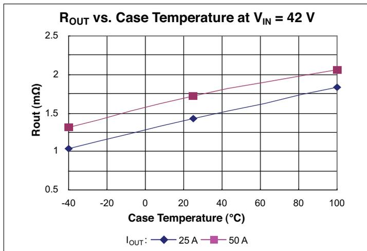
Figure 6 — R<sub>OUT</sub> vs. temperature
