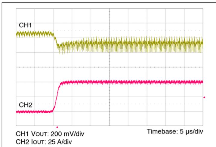
Figure 15 — 0 A – 50 A transient response:  $C_{IN} = 100 \mu$ F, no external  $C_{OUT}$
