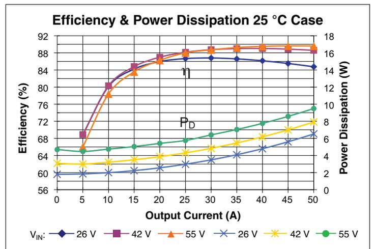
Figure 4 — Efficiency and power dissipation at  $25^\circ\text{C}$
