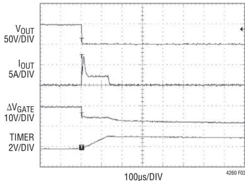
Figure 3. Short-Circuit Waveforms
