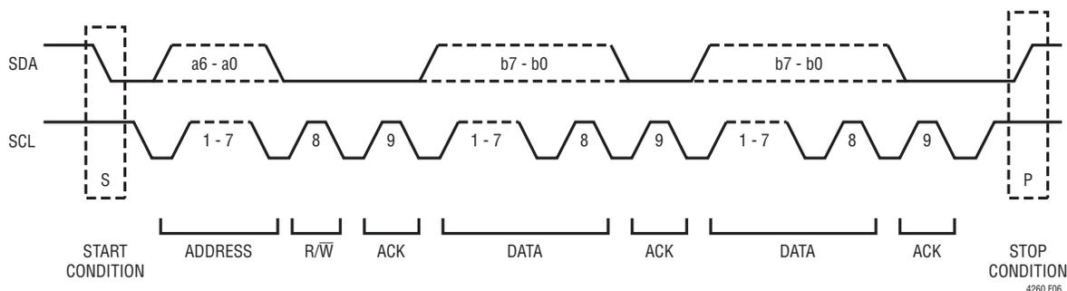
Figure 6. Data Transfer Over I<sup>2</sup>C or SMBus
