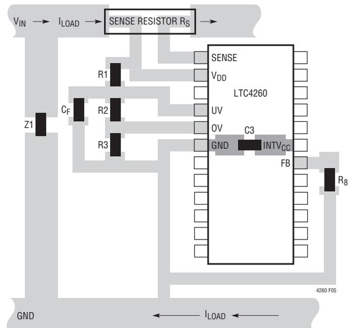
Figure 5. Recommended Layout for R1, R2, R3, R8, C<sub>F</sub>, C3, Z1 and R<sub>S</sub>
