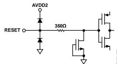
Figure 29. Equivalent RESET Input Circuit
