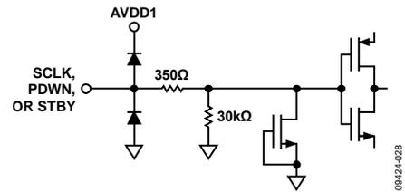
Figure 28. Equivalent SCLK, PDWN, or STBY Input Circuit
