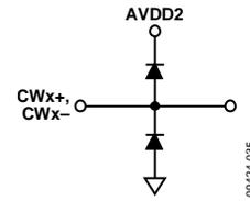
Figure 35. Equivalent CWI±, CWQ± Output Circuit
