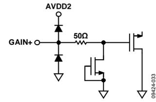
Figure 33. Equivalent GAIN+ Input Circuit
