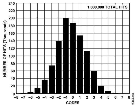
Figure 8. Output-Referred Noise Histogram, GAIN+ = 1.6 V
