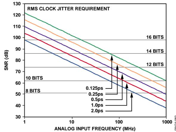
Figure 55. Ideal SNR vs. Input Frequency and Jitter
