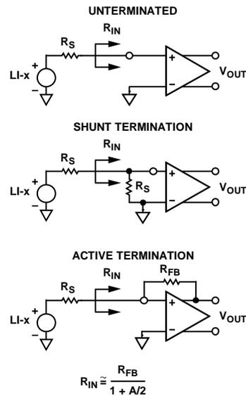
Figure 44. Input Configurations
