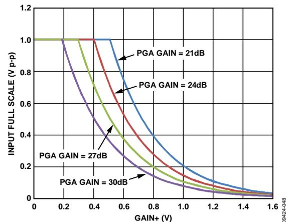
Figure 40. LNA with 15.6 dB Gain Setting/VGA Full-Scale Limitations
