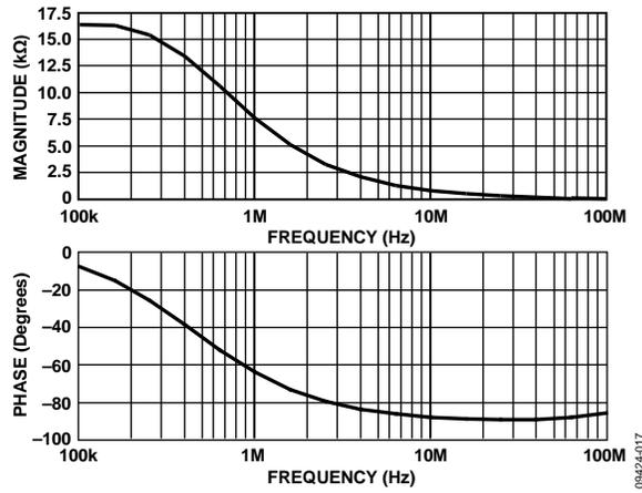
Figure 18. LNA Input Impedance Magnitude and Phase, Underterminated
