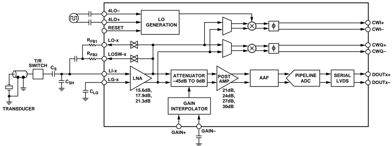
Figure 38. Simplified Block Diagram of a Single Channel
