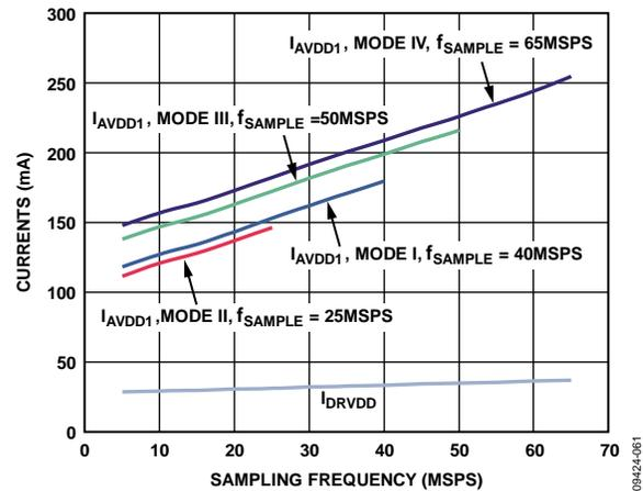
Figure 56. Supply Current vs.  $f_{SAMPLE}$  for  $f_{IN} = 5$  MHz
