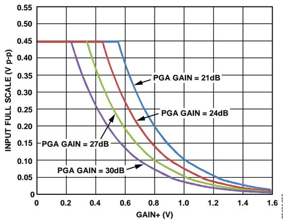
Figure 42. LNA with 21.3 dB Gain Setting/VGA Full-Scale Limitations
