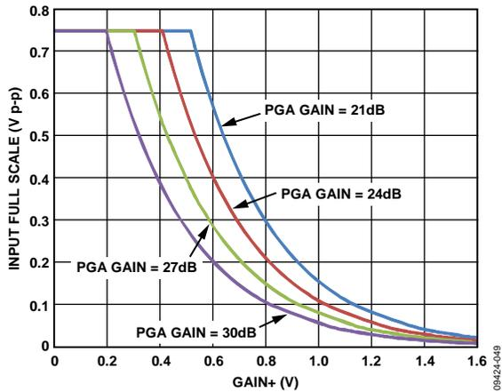
Figure 41. LNA with 17.9 dB Gain Setting/VGA Full-Scale Limitations
