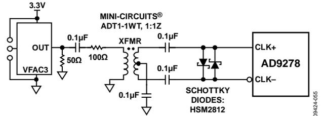
Figure 50. Transformer-Coupled Differential Clock
