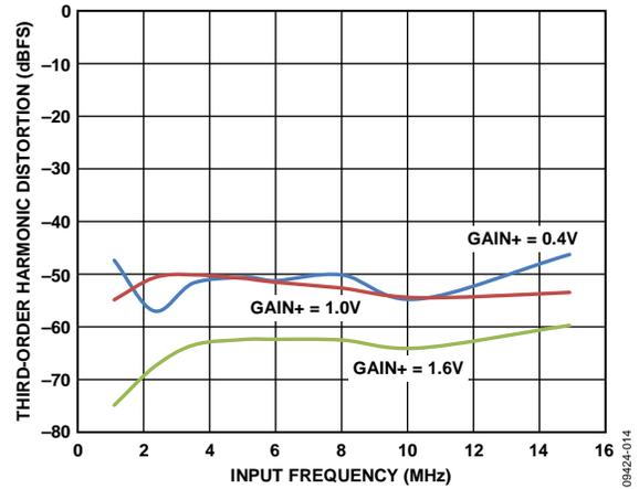
Figure 15. Third-Order Harmonic Distortion vs. Frequency, AOUT = -1.0 dBFS
