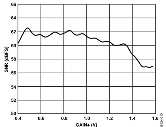
Figure 11. SNR vs. GAIN+, AOUT = -1.0 dBFS
