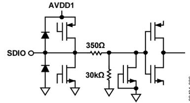
Figure 26. Equivalent SDIO Input Circuit
