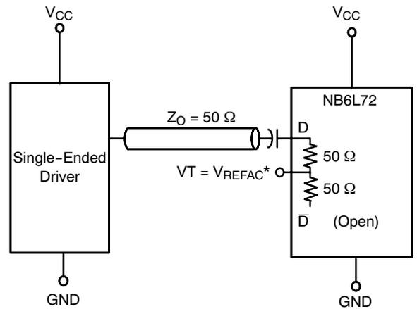
Figure 14. Capacitor-Coupled Single-Ended Interface
