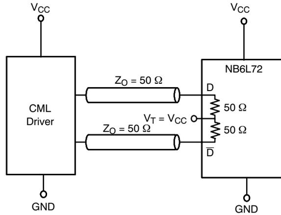
Figure 12. Standard 50  $\Omega$  Load CML Interface
