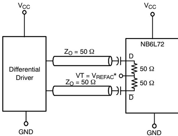
Figure 13. Capacitor-Coupled Differential Interface
