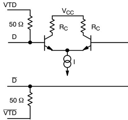
Figure 3. Input Structure
