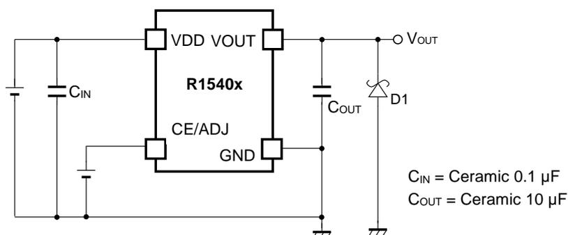
R1540x Typical Application for IC Chip Breakdown Prevention
