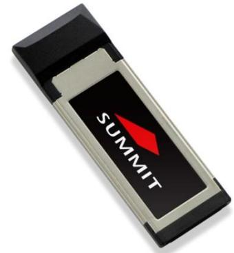
When operating on channels in the UNII-2 and UNII-2 Extended bands that are in the 5GHz portion of the frequency spectrum and are subject to Dynamic Frequency Selection requirements, the SDC-EC25N fully conforms to applicable regulatory requirements. In the event that specified types of radar are detected by the network infrastructure, the SDC-EC25N fully conforms with commands from the infrastructure for radar avoidance.
