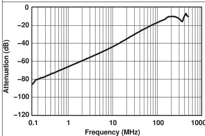
Figure 9. OFF Isolation and Crosstalk (V<sub>+</sub> = 5 V)
