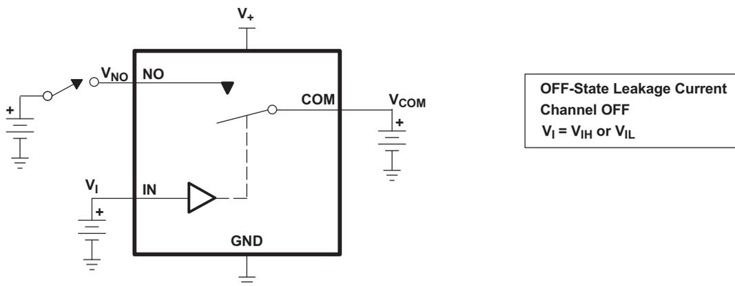
Figure 12. OFF-State Leakage Current ( $I_{COM(OFF)}$ ,  $I_{NC(OFF)}$ ,  $I_{COM(PWROFF)}$ ,  $I_{NC(PWR(F))}$ )
