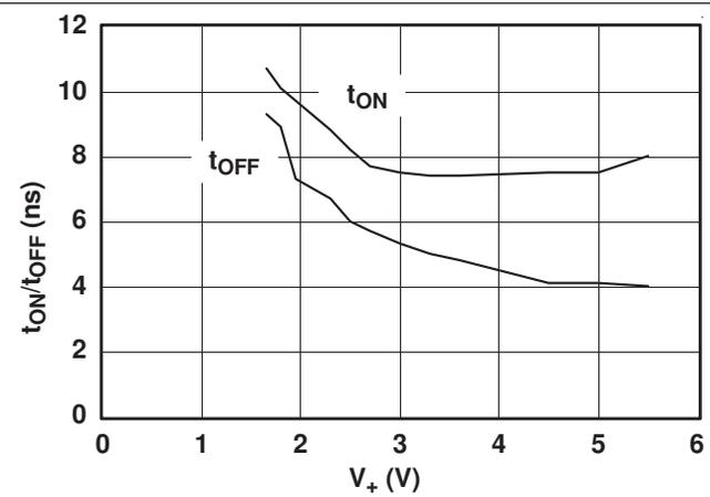
Figure 6.  $t_{ON}$  and  $t_{OFF}$  vs Supply Voltage
