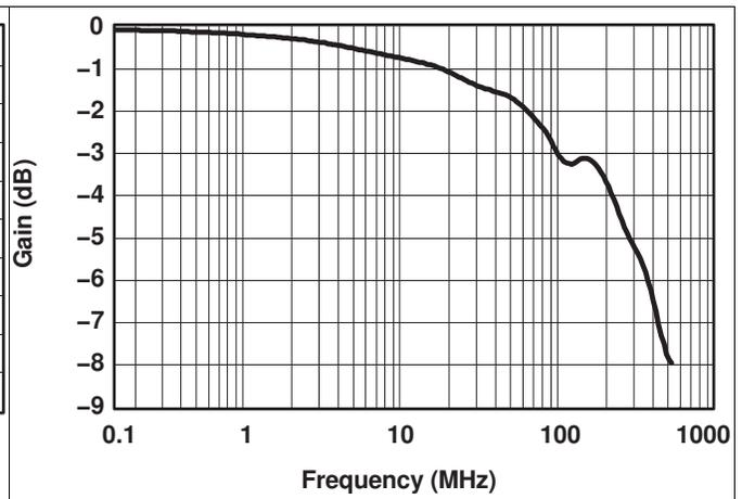
Figure 8. Bandwidth (V<sub>+</sub> = 5 V)
