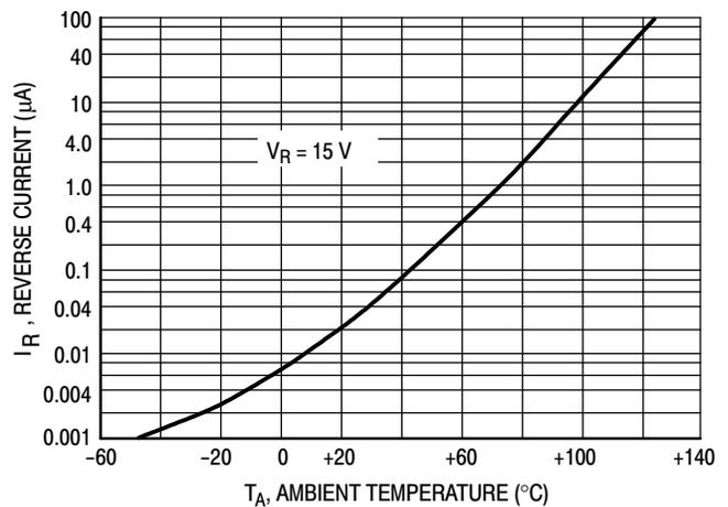
Figure 4. Leakage Current
