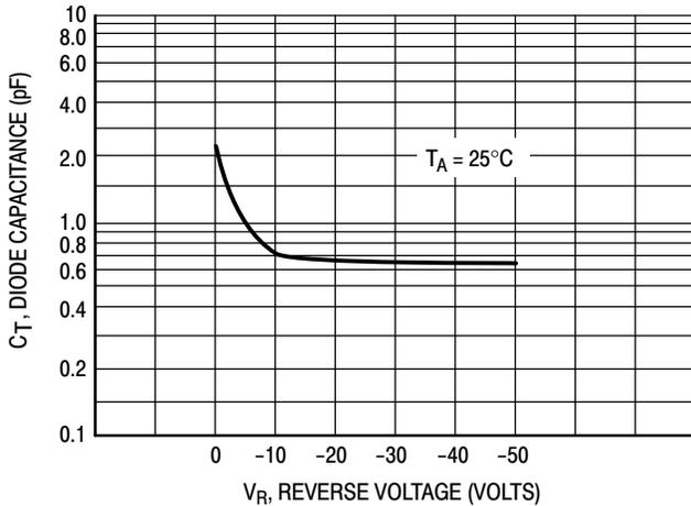
Figure 3. Diode Capacitance
