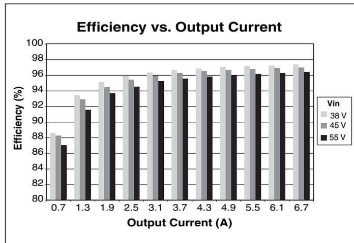
Figure 7 — Efficiency vs. output current at 36 Vf
