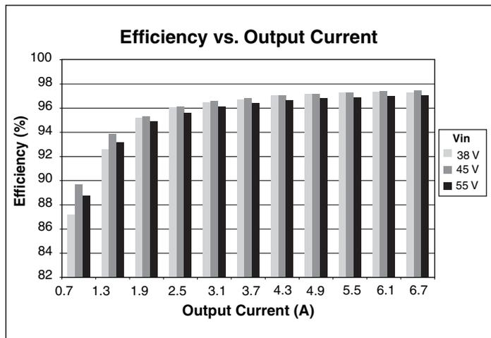
Figure 6 — Efficiency vs. output current at 48 Vf
