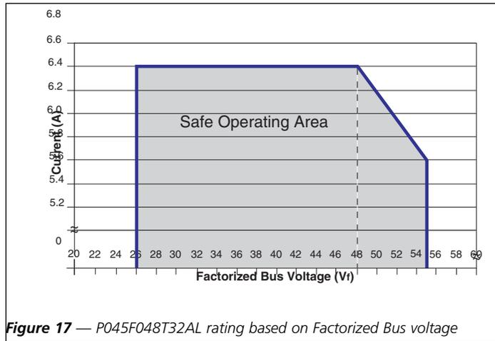
Figure 17 — P045F048T32AL rating based on Factorized Bus voltage
