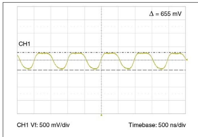
Figure 14 — Output ripple full load 10μF bypass capacitance
