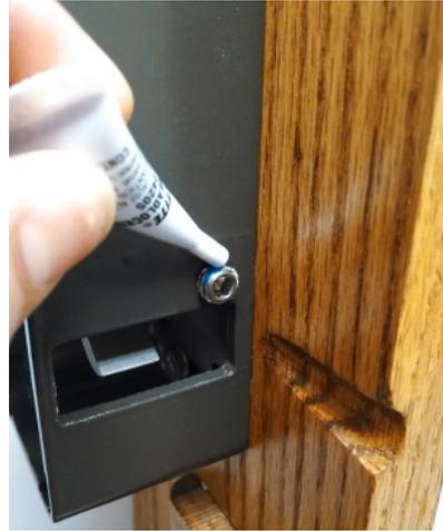
9. Tighten the two (2) set screws two full revolutions. The face of the set screw should be flush with the side of the interlock housing. If it is not, adjust the set screw to achieve this. Wipe off excess Loctite with a rag.
