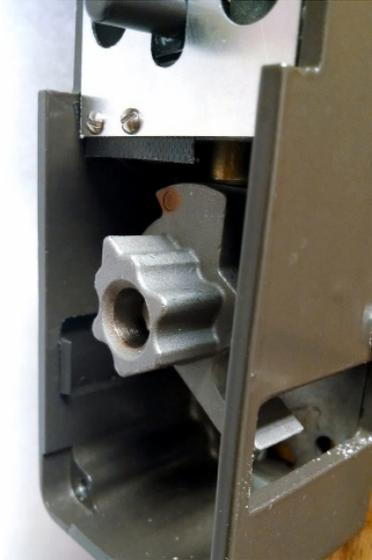
7. Insert new metal cam in the same orientation as noted in step 4. To start the insertion, make sure the arrow on the cam is pointing toward the center of the unit (toward the solenoid).
