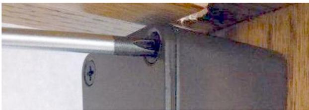
2. Hold the locking pin away from the plastic cam, and rotate the cam back and forth a few times to get a feel for proper operation of the cam. Some force will be required.
