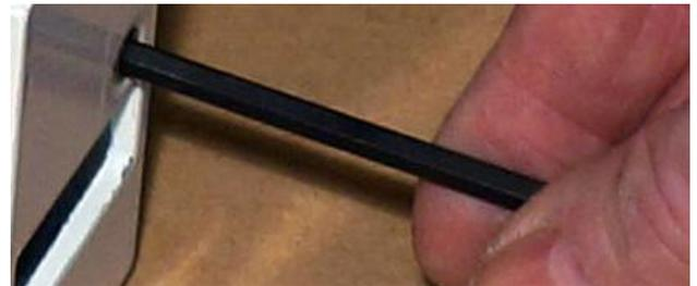
10. Hold up on the locking pin and rotate the new metal cam back and forth a few times to ensure smooth operation and no binding. The operation should feel like what was noted in step 2.
