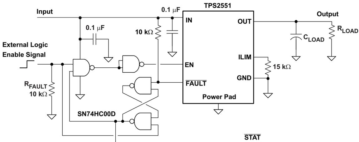
Figure 24. Overcurrent Latch-Off Using a Quad-NAND Gate
