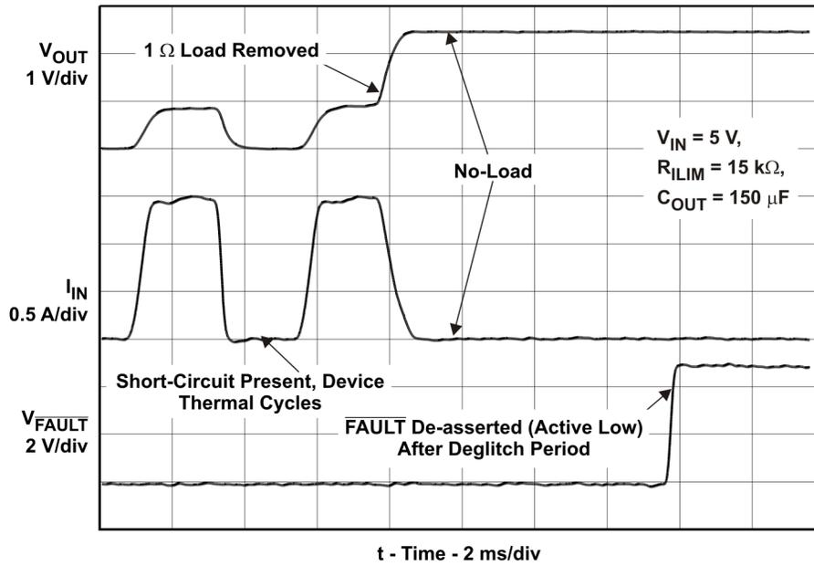
Figure 13. 1 $\Omega$  to No Load Transient Response
