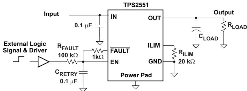
Figure 23. Auto-Retry Functionality With External EN Signal
