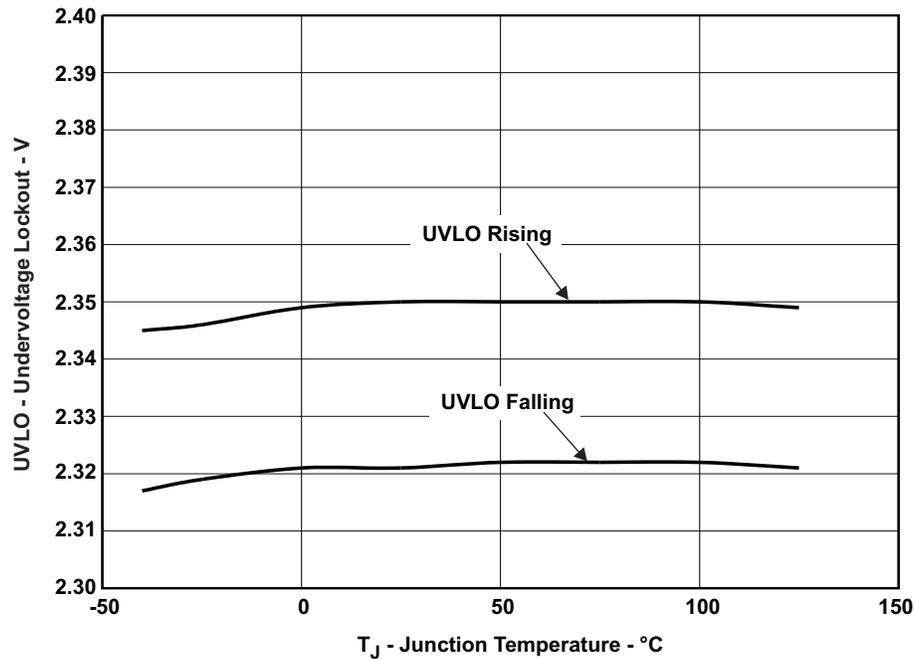
Figure 16. UVLO – Undervoltage Lockout – V
