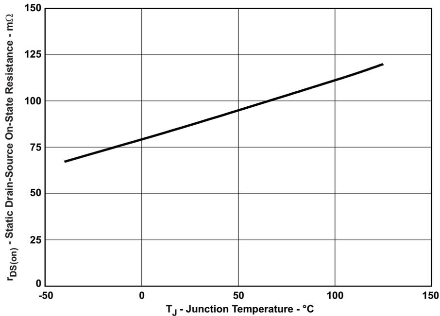
Figure 20. MOSFET r<sub>DS(on)</sub> Vs. Junction Temperature
