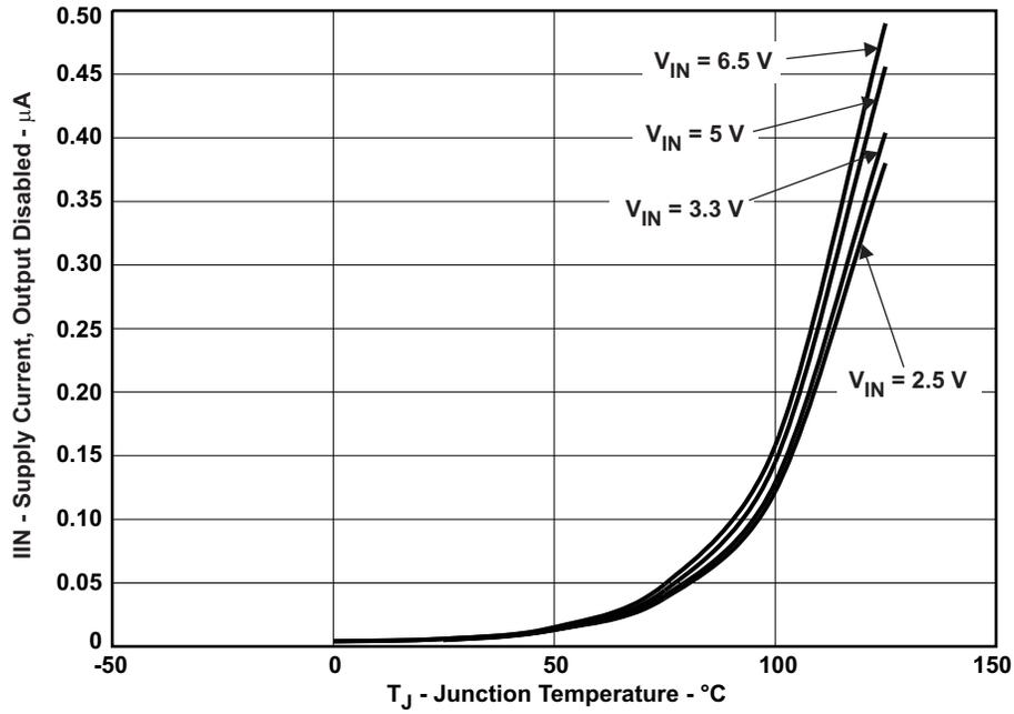
Figure 17.  $I_{IN}$  – Supply Current, Output Disabled –  $\mu A$
