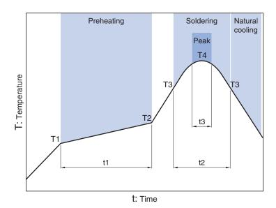
Preheating Soldering Peak Temp. Time Temp. Time Time Temp. T2 T4 t3 150°C 180°C 60 to 120s 230°C 30s 250°C 5s
