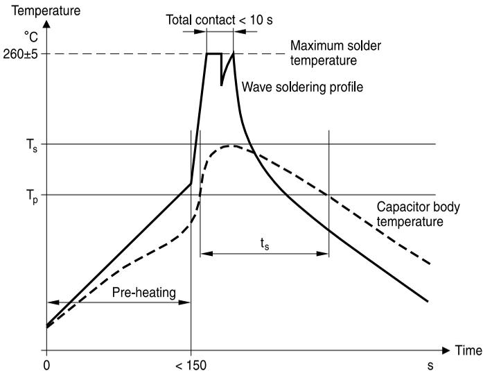
$T_s$ : Capacitor body maximum temperature at wave soldering
