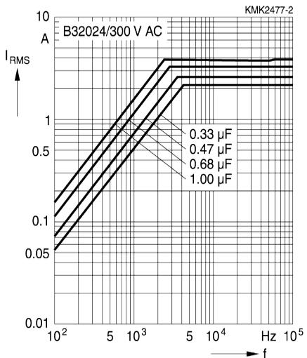
**Permissible AC current  $I_{RMS}$  versus frequency  $f$  (for sinusoidal waveforms  $T_A \leq 100^\circ\text{C}$  and  $\Delta ESR < 100\%$  from receipt condition)**
