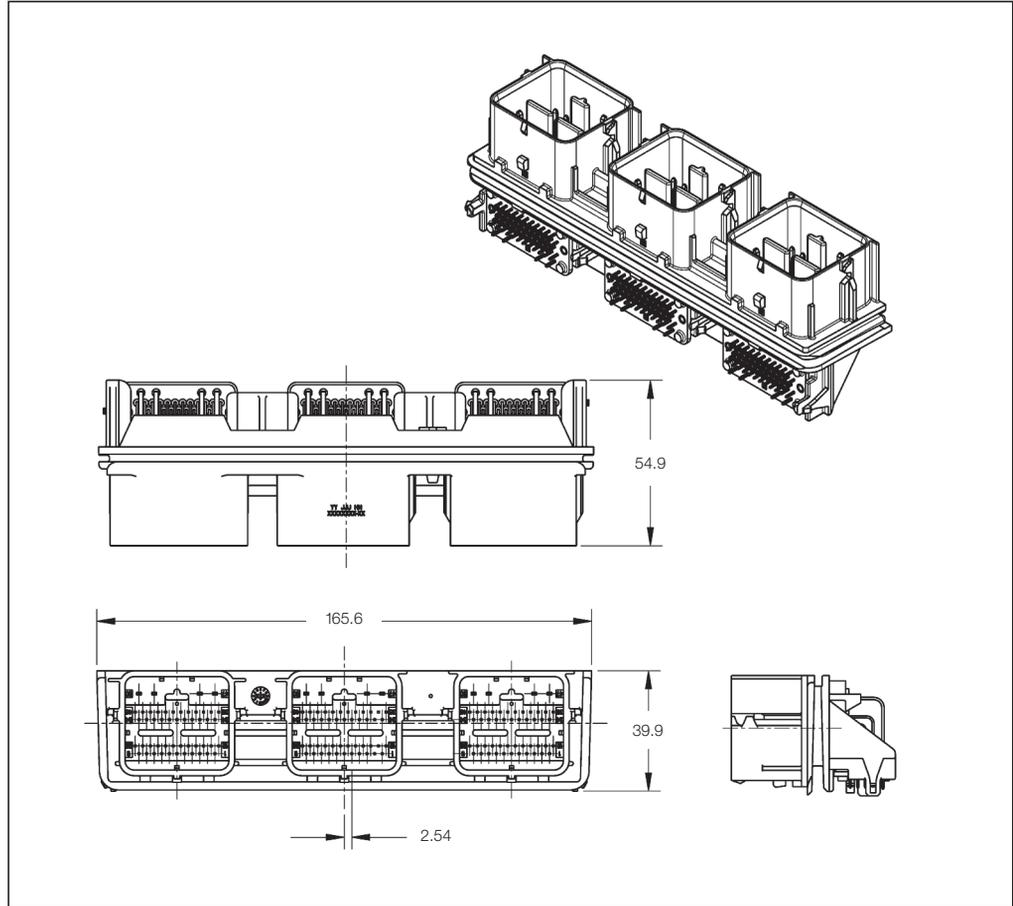
**Sealed Printed Circuit Board Headers**
