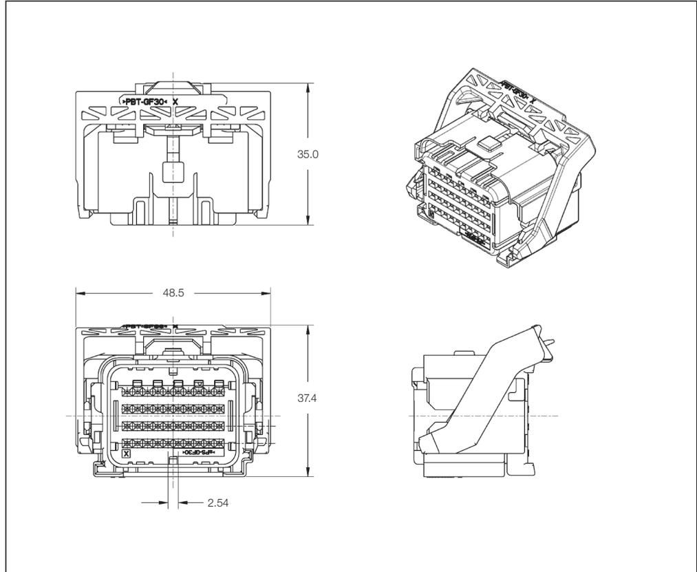
**Sealed Receptacle Housings 4-Row with Standard Lever**
