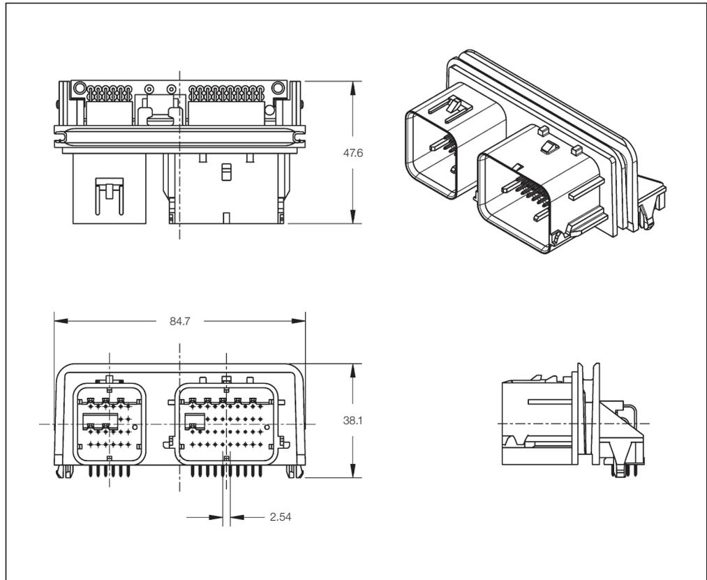
**Sealed Printed Circuit Board Headers**
