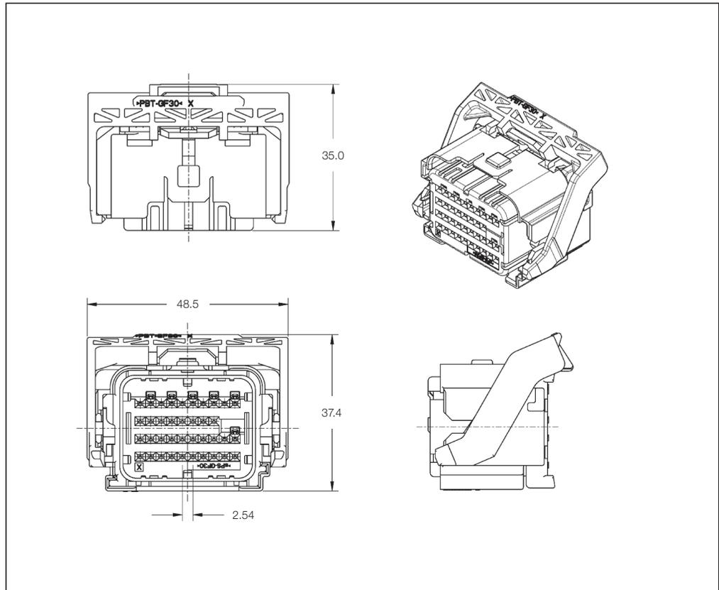
**Sealed Receptacle Housings 4-Rows with Low Profile Lever**
