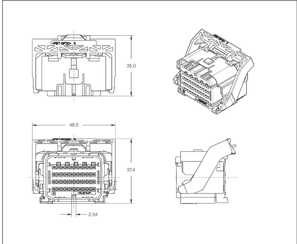
**Sealed Receptacle Housings 4-Row with Low Profile Lever**
