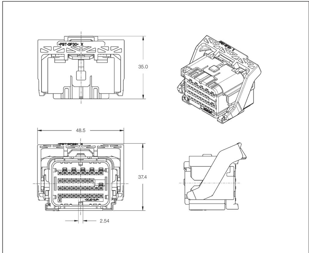
**Sealed Receptacle Housings 4-Rows with Standard Lever**
