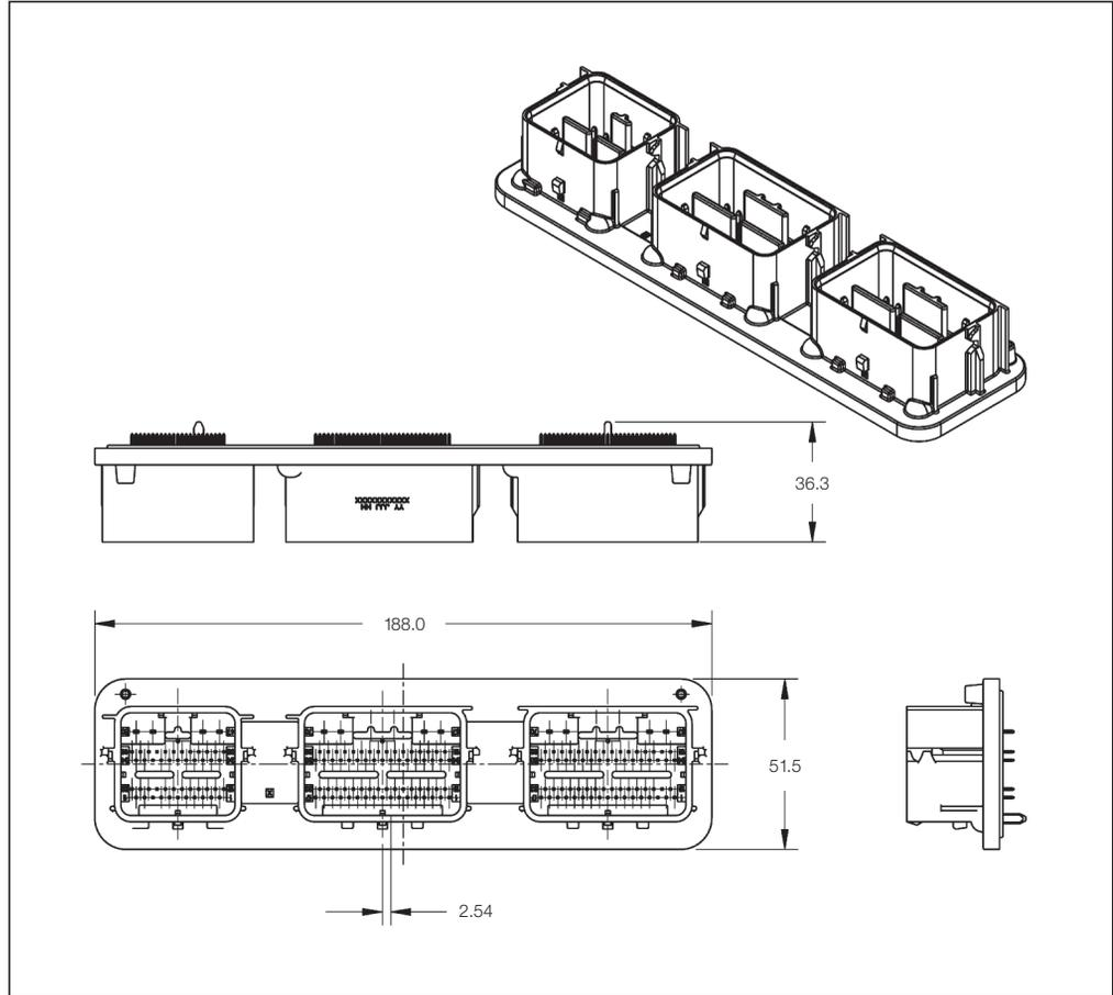
**Sealed Printed Circuit Board Headers**
