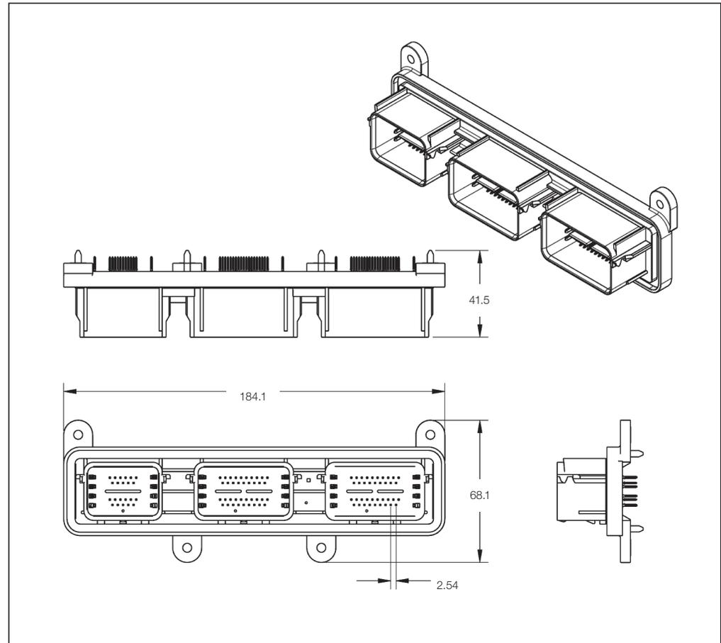
**Sealed Printed Circuit Board Headers**
