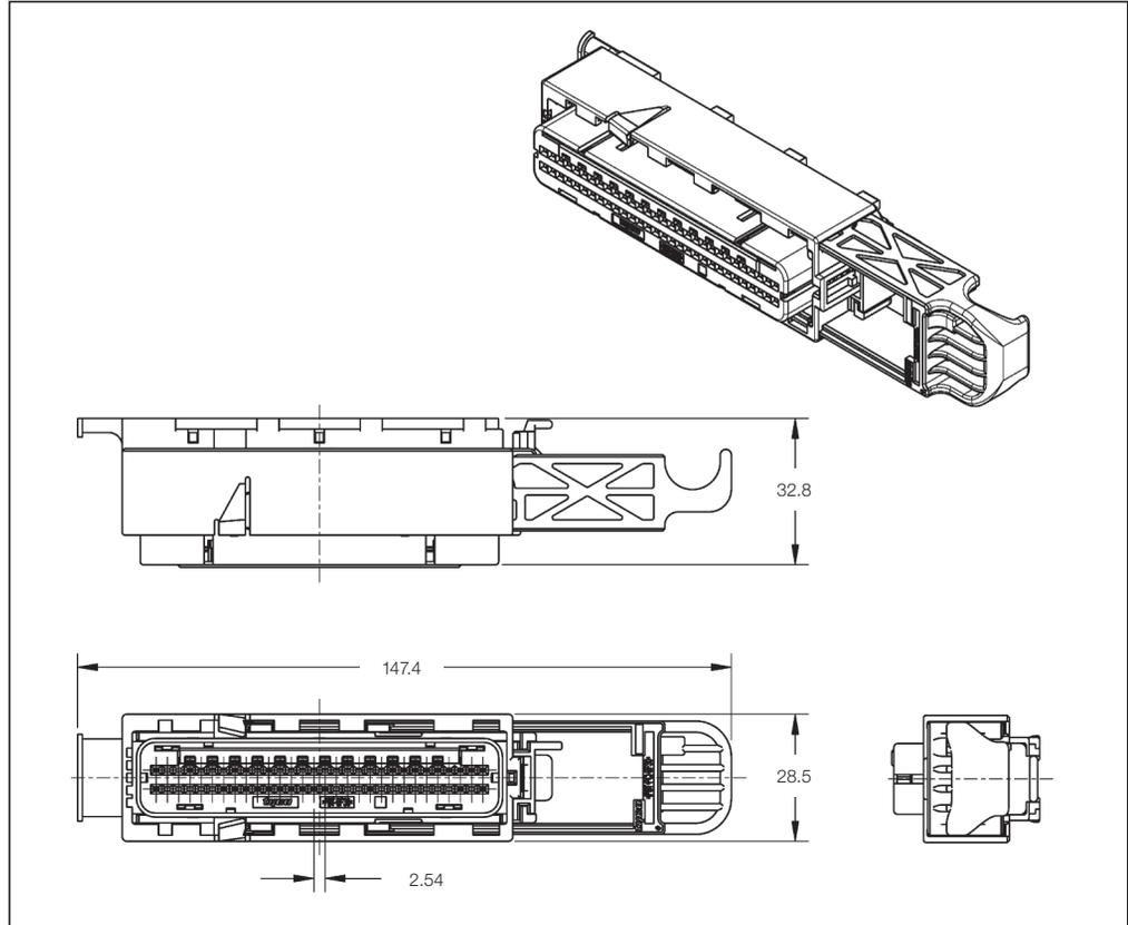
**Sealed Receptacle Housings – Multiple Rows with Shorting Bars**
