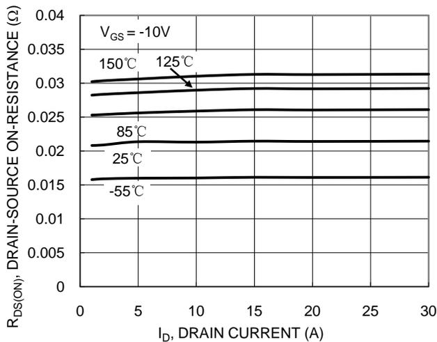
Figure 17. Typical On-Resistance vs. Drain Current and Temperature
