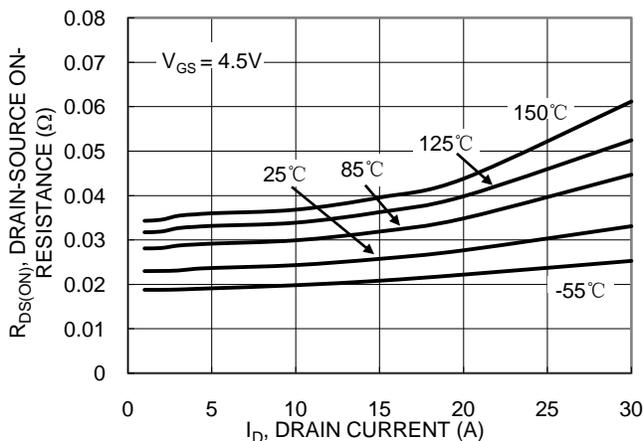
Figure 5. Typical On-Resistance vs. Drain Current and Temperature
