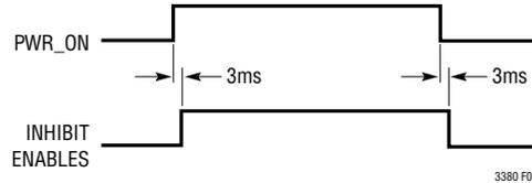
Figure 6. Power Up and Down with PWR\_ON
