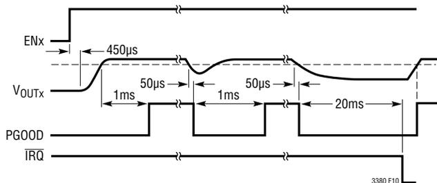
Figure 10. Output Low Voltage PGOOD and  $\overline{\text{IRQ}}$  Timing
