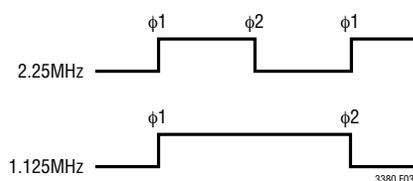
Figure 3. Phase Settings Full- and Half-Speed Buck Clock
