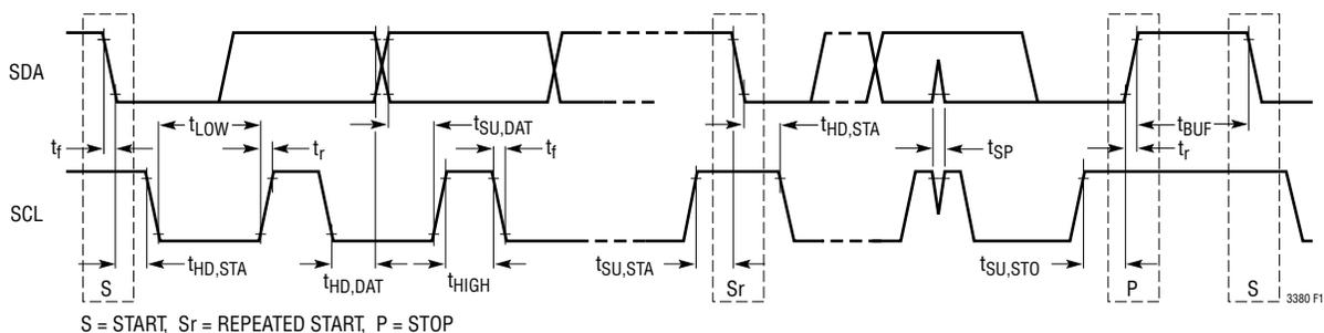
**Figure 11. LT3380 I<sup>2</sup>C Serial Port Timing**
