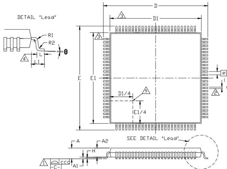
**Figure 3 - 100 Pin TQFP Package Outline**
