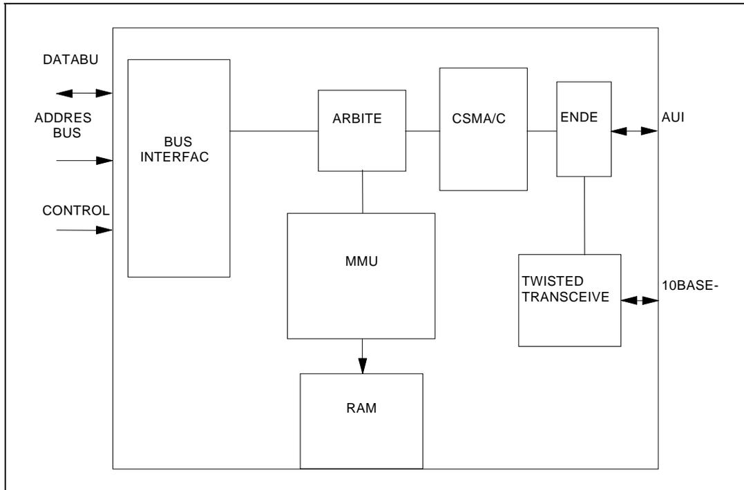
Figure 1 - LAN91C96i Internal Block Diagram
