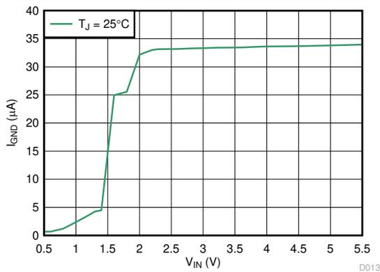
**Figure 6-3. Ground Pin Current vs  $V_{IN}$**
