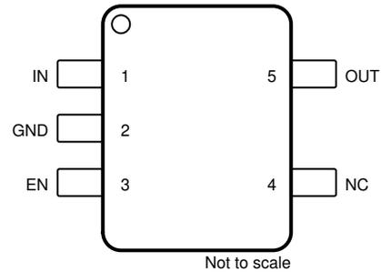
Figure 5-2. DBV Package, 5-Pin SOT-23, Top View
