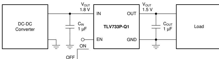
Figure 8-2. DC-DC Converter Post Regulation
