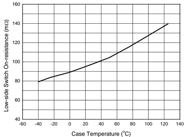
**Performance Characteristics** (Cont.  $V_{IN}=12V$ ,  $V_{OUT}=3.3V$ , unless otherwise noted.)
