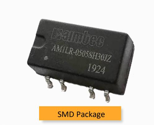
The AM1LR-JZ is a 1W SMD DC/DC converter that offers great cost savings thanks to an improved manufacturing process. It also features excellent reliability and performance while offering a standard input voltage range of 5-24VDC as well as an output voltage of 3.3-15V. This compact SMD design will surely benefit your new system design.
