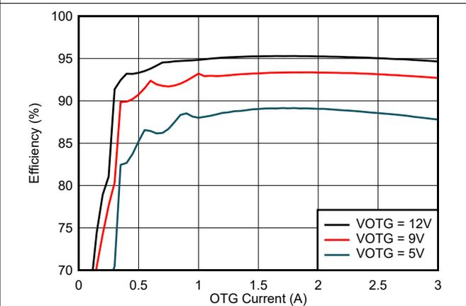
$V_{BAT} = 16.8\text{V}$ ,  $F_{sw} = 1.5 \text{ MHz}$  with  $L1 = 1 \mu\text{H}$ , PFM disabled
