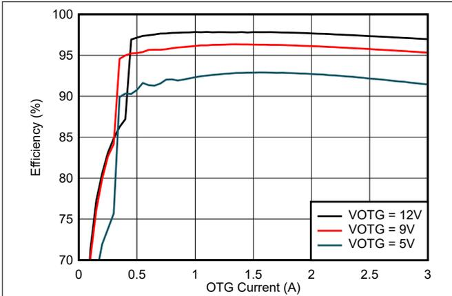
$V_{BAT} = 12.6\text{V}$ ,  $F_{sw} = 750 \text{ kHz}$  with  $L2 = 2.2 \mu\text{H}$ , PFM disabled
