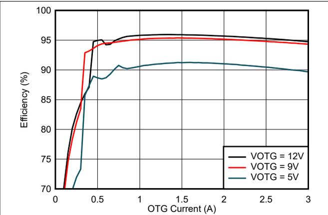
$V_{BAT} = 12.6\text{V}$ ,  $F_{sw} = 1.5 \text{ MHz}$  with  $L1 = 1 \mu\text{H}$ , PFM disabled
