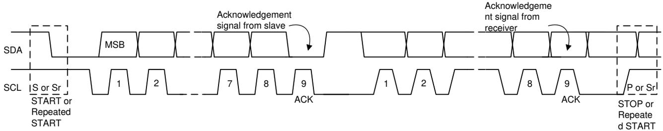
**Figure 8-17. Data Transfer on the I<sup>2</sup>C Bus**
