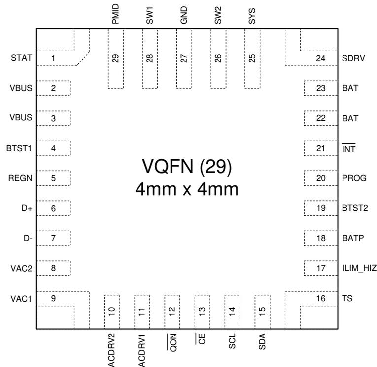
**Figure 6-1. RQM Package 29-Pin VQFN Top View**
