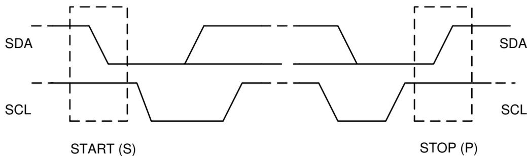
**Figure 8-16. START and STOP Conditions on the I<sup>2</sup>C Bus**
