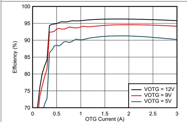
$V_{BAT} = 16.8\text{V}$ ,  $F_{sw} = 750 \text{ kHz}$  with  $L2 = 2.2 \mu\text{H}$ , PFM disabled
