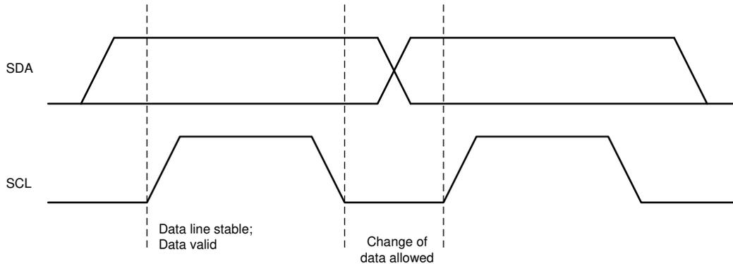
**Figure 8-15. Bit Transfers on the I<sup>2</sup>C Bus**
