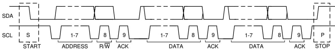
**Figure 8-19. Complete Data Transfer on the I<sup>2</sup>C Bus**
