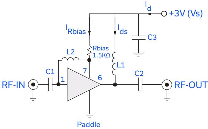
Fig 3. Recommended Application Circuit
