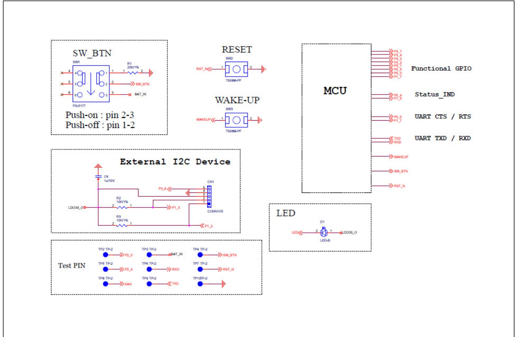
FIGURE 2-11: RN4678 REFERENCE CIRCUIT
