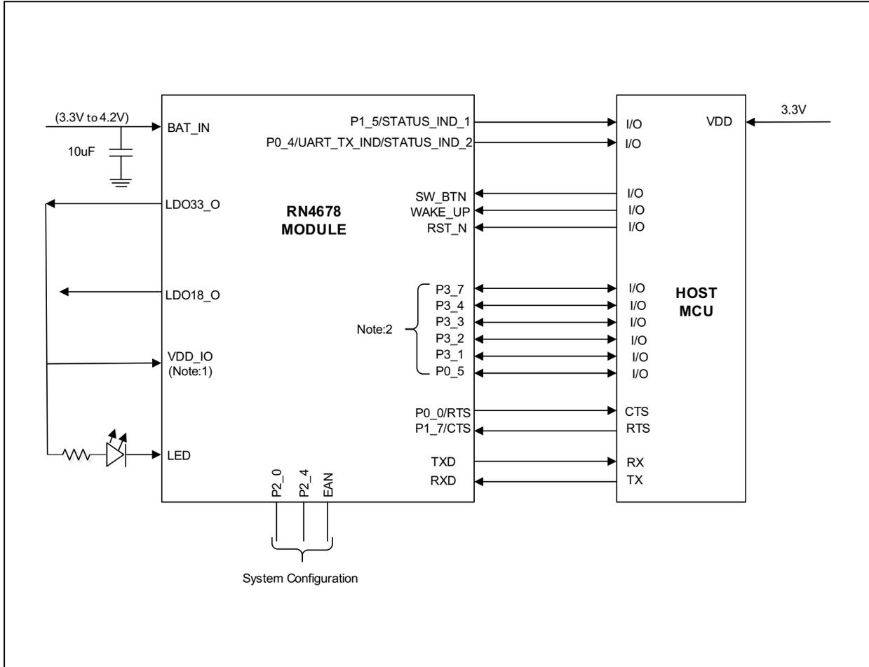
**Note 1:** Ensure that VDD\_IO and MCU VDD voltages are compatible.
