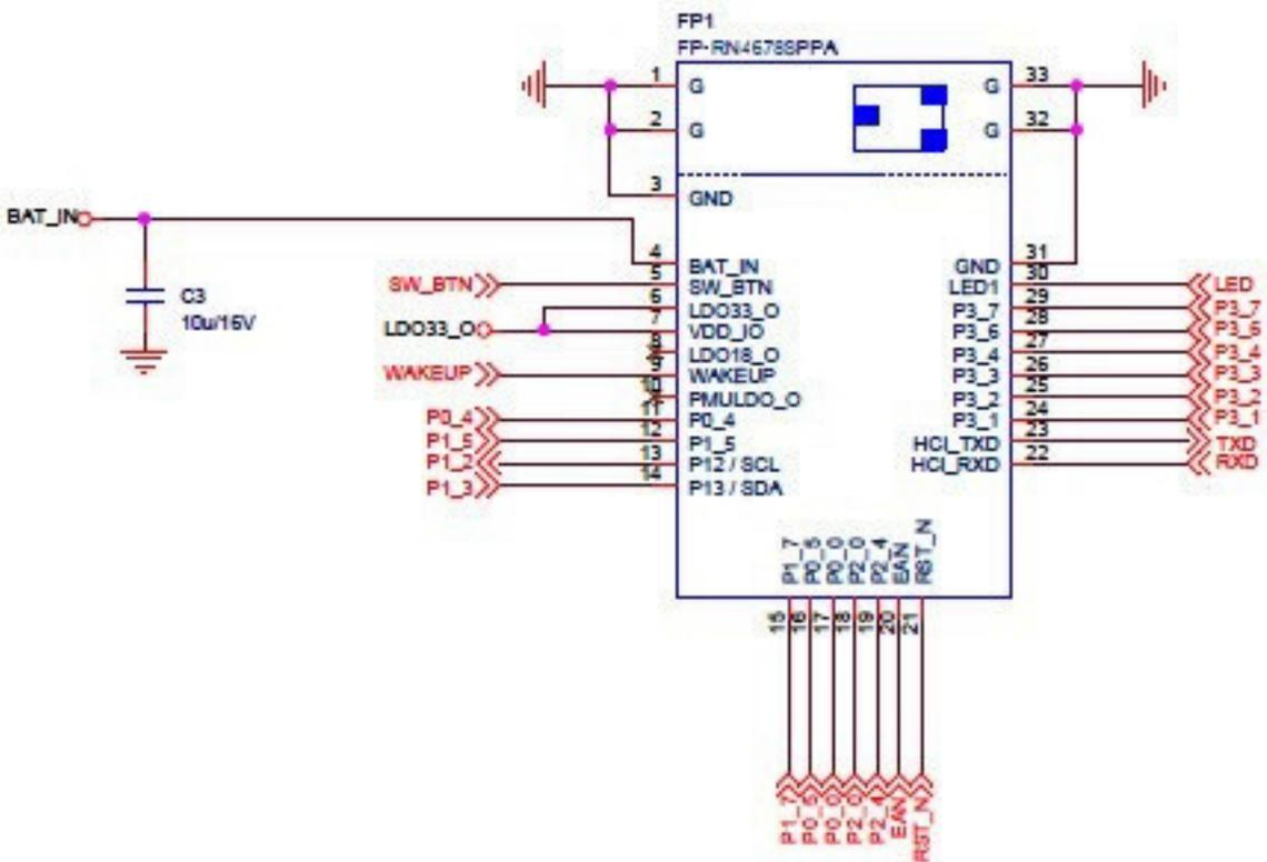
FIGURE 2-12: RN4678 REFERENCE CIRCUIT
