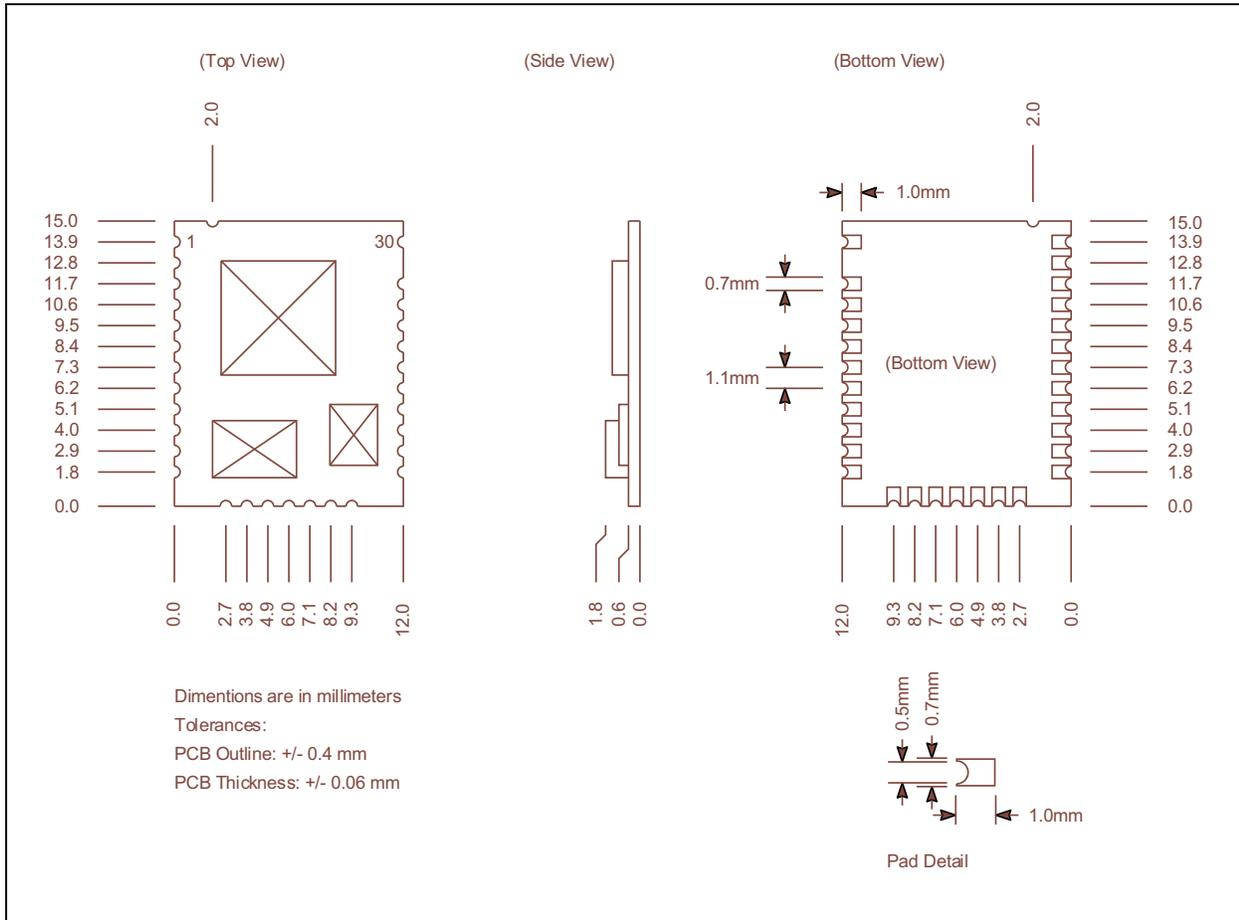
Figure 5-5 illustrates the recommended host PCB footprint.
