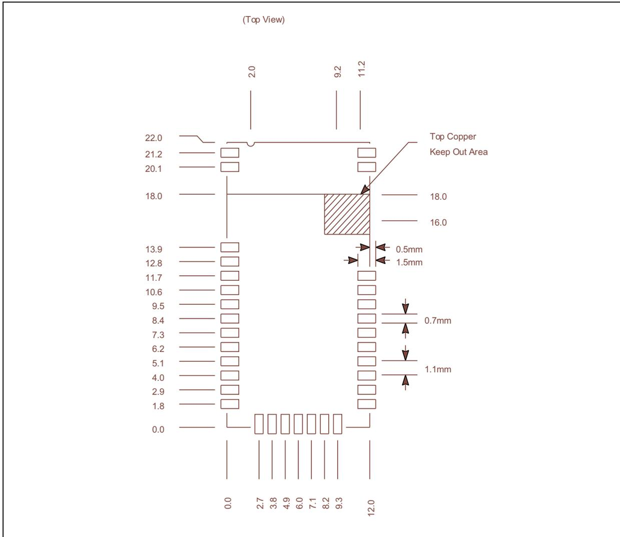
Figure 5-3 illustrates the recommendations for mounting the RN4678 on the host PCB, and also shows the minimum ground plane area to the left and right of the module for the best antenna performance.
