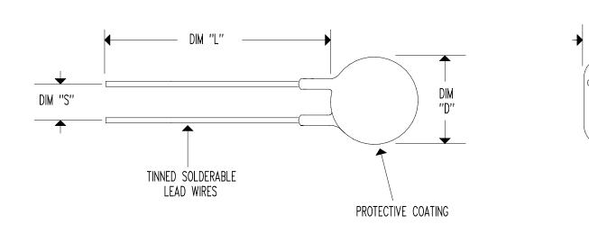
RESISTANCE @  $+25^{\circ}C = 5 \Omega \pm 20^{\%}$  MAXIMUM STEADY STATE CURRENT (Imax) = 8 AMPS
