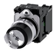
RONIS key-operated switch, 22 mm, round, metal, shiny, lock number SB30, with 2 keys, 2 switch positions O-I, latching, actuating angle 90°, 10:30h/13:30h, key removal O+I, with holder, 1 NO, screw terminal, possible special locks: SB31, 421, 455
