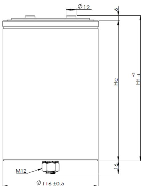
Figure 4: - B25620C -  $\varnothing$  116mm
