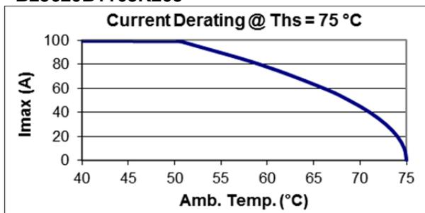
Current derating graphs are based on typical values. Graphs for capacitors rated 1320 / 1500/2000 U<sub>NDC</sub> are available upon request.
