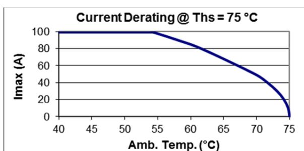
2.2 Current derating graphs for capacitors 900 V<sub>RDC</sub>
