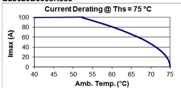
**2.3 Current derating graphs for capacitors 1100 V<sub>RDC</sub>**
