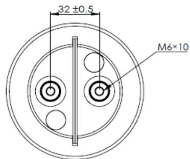
Figure 3: - B25620B -  $\varnothing$  116mm
