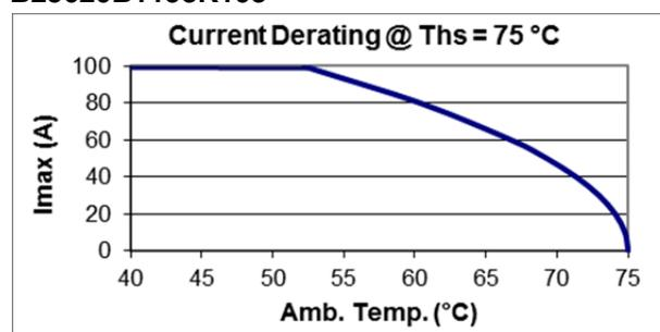
**2.4 Current derating graphs for capacitors 1200 V<sub>RDC</sub>**
