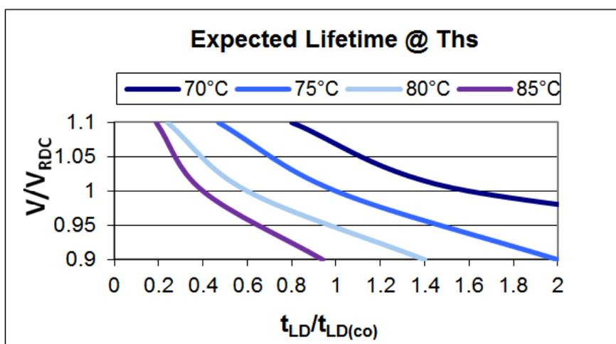
Service life t<sub>LD</sub> at different hotspot temperature (Θ<sub>hs</sub>) and voltage V
