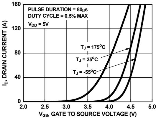
Figure 7. Transfer Characteristics
