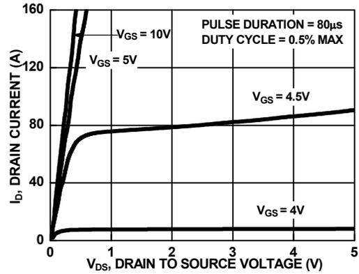
Figure 8. Saturation Characteristics
