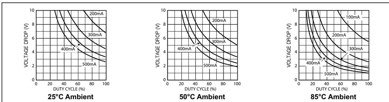
**FIGURE 4-4:** MIC5219-x.xYMM (MSOP-8) on 1-Inch<sup>2</sup> Copper Cladding.
