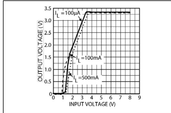
**FIGURE 2-12:** Dropout Characteristics.
