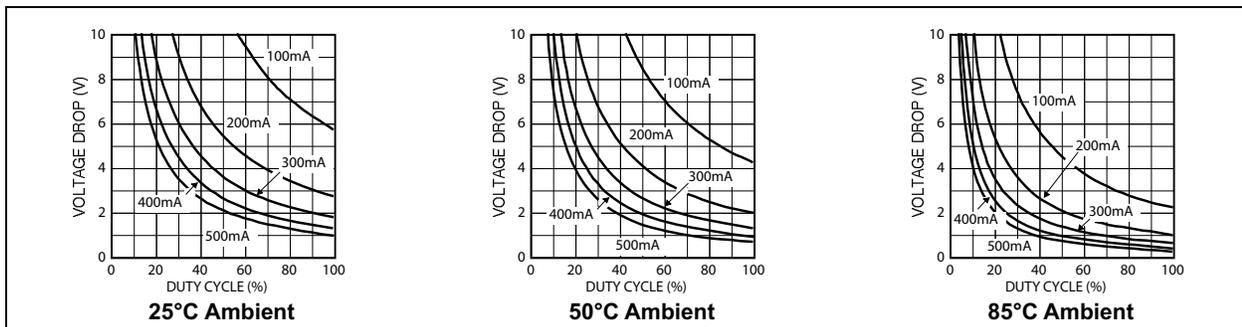
**FIGURE 4-2:** MIC5219-x.xYM5 (SOT23-5) on 1-Inch<sup>2</sup> Copper Cladding.
