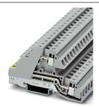
Installation ground terminal block, Screw connection, cross section: 0.2 mm² - 10 mm², AWG: 24 - 8, width: 8.2 mm, color: gray, mounting type: NS 35/7,5, NS 35/15
