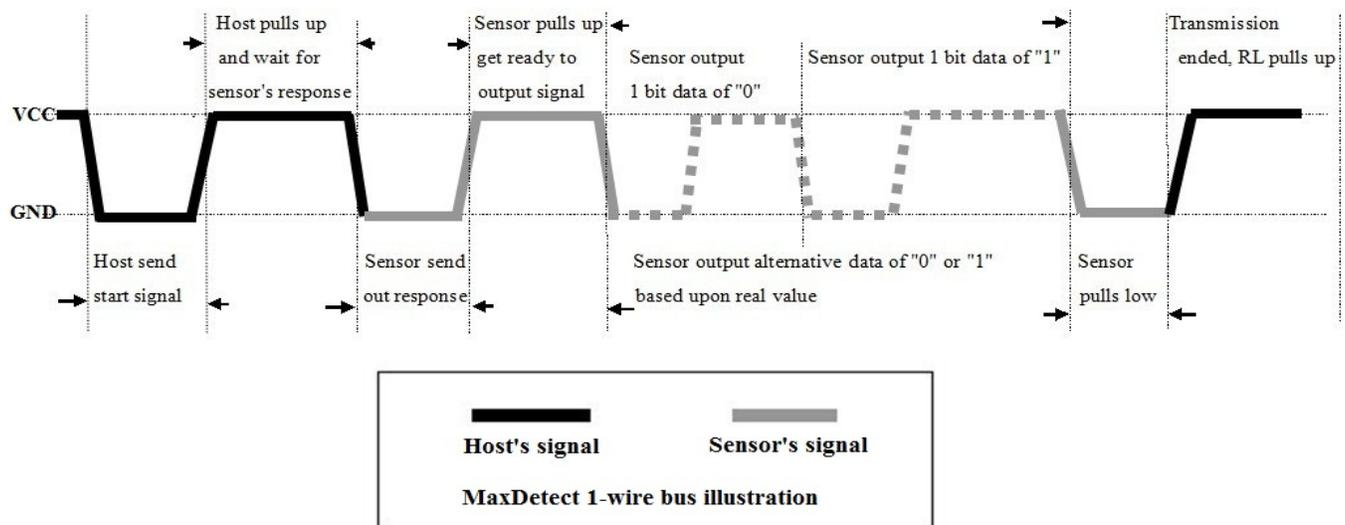
1) Step 1: MCU send out start signal to RHT03 and RHT03 send response signal to MCU
