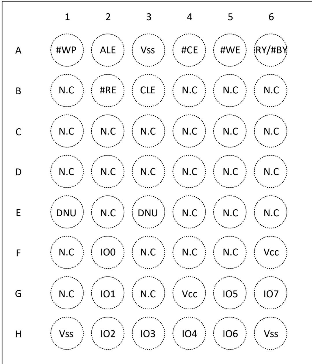
Figure 3-2 Pin Assignment 48-ball VFBGA (Package code D)
