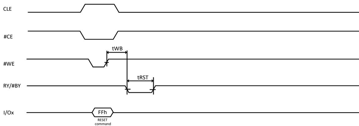
Figure 9-19 Reset Operation
