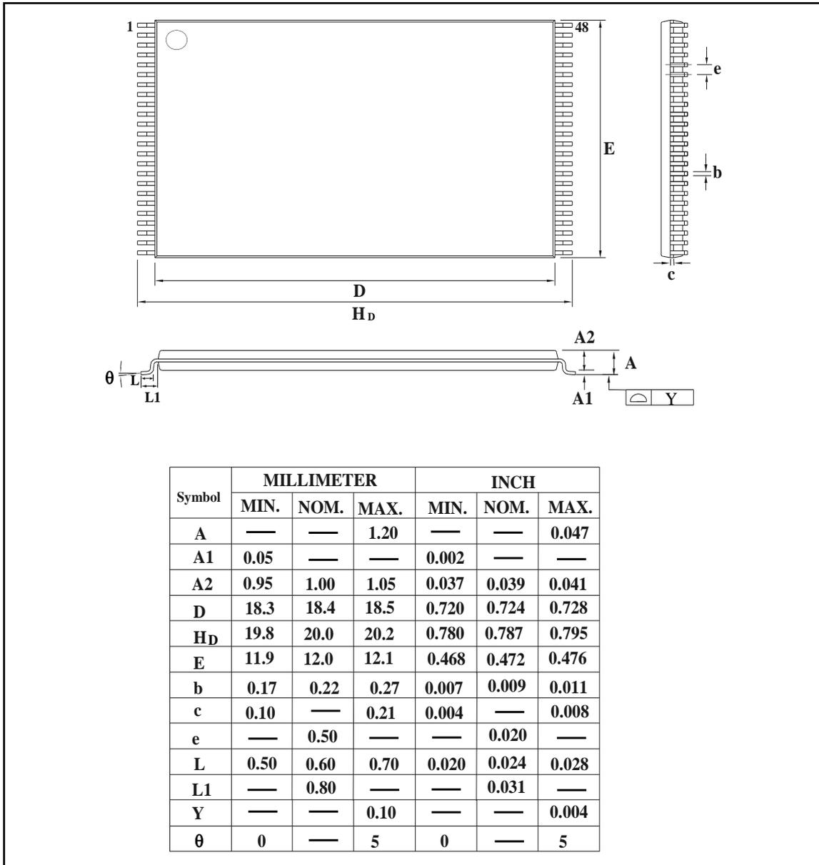
Figure 13-1 TSOP 48-PIN 12X20mm
