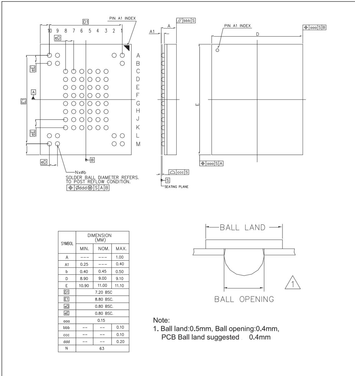
Figure 13-3 Fine-Pitch Ball Grid Array 63-Ball
