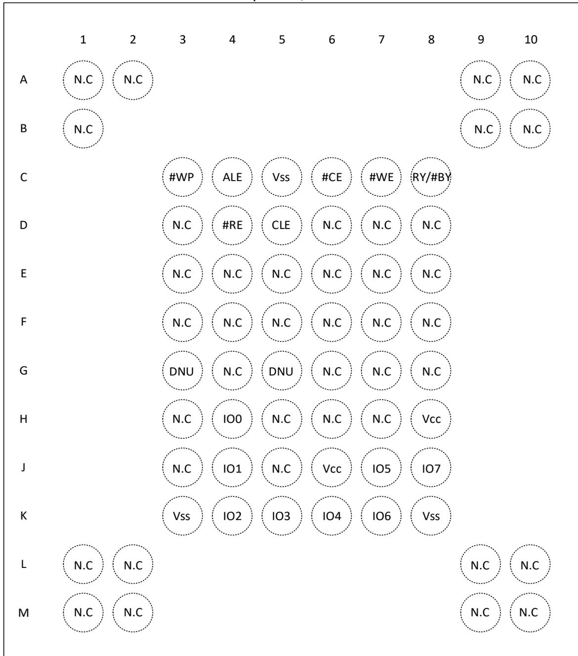
Figure 3-3 Pin Assignment 63-ball VFBGA (Package code B)
