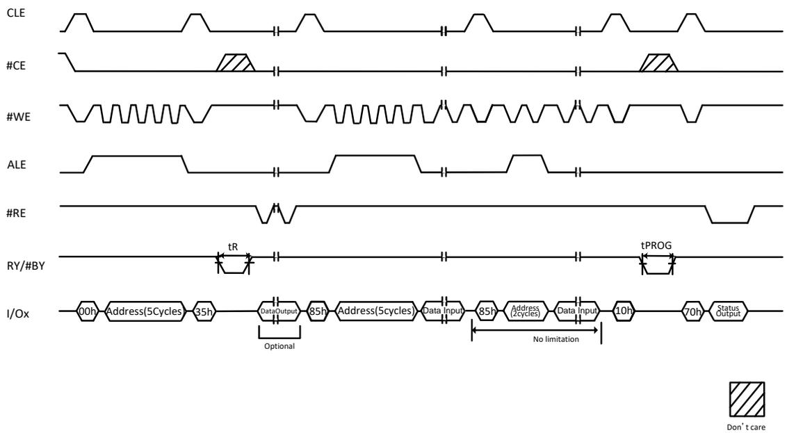
Figure 9-13 Copy Back Operation with Random Data Input
