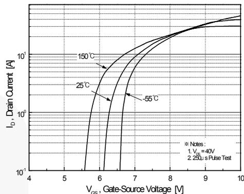
Figure 2. Transfer Characteristics
