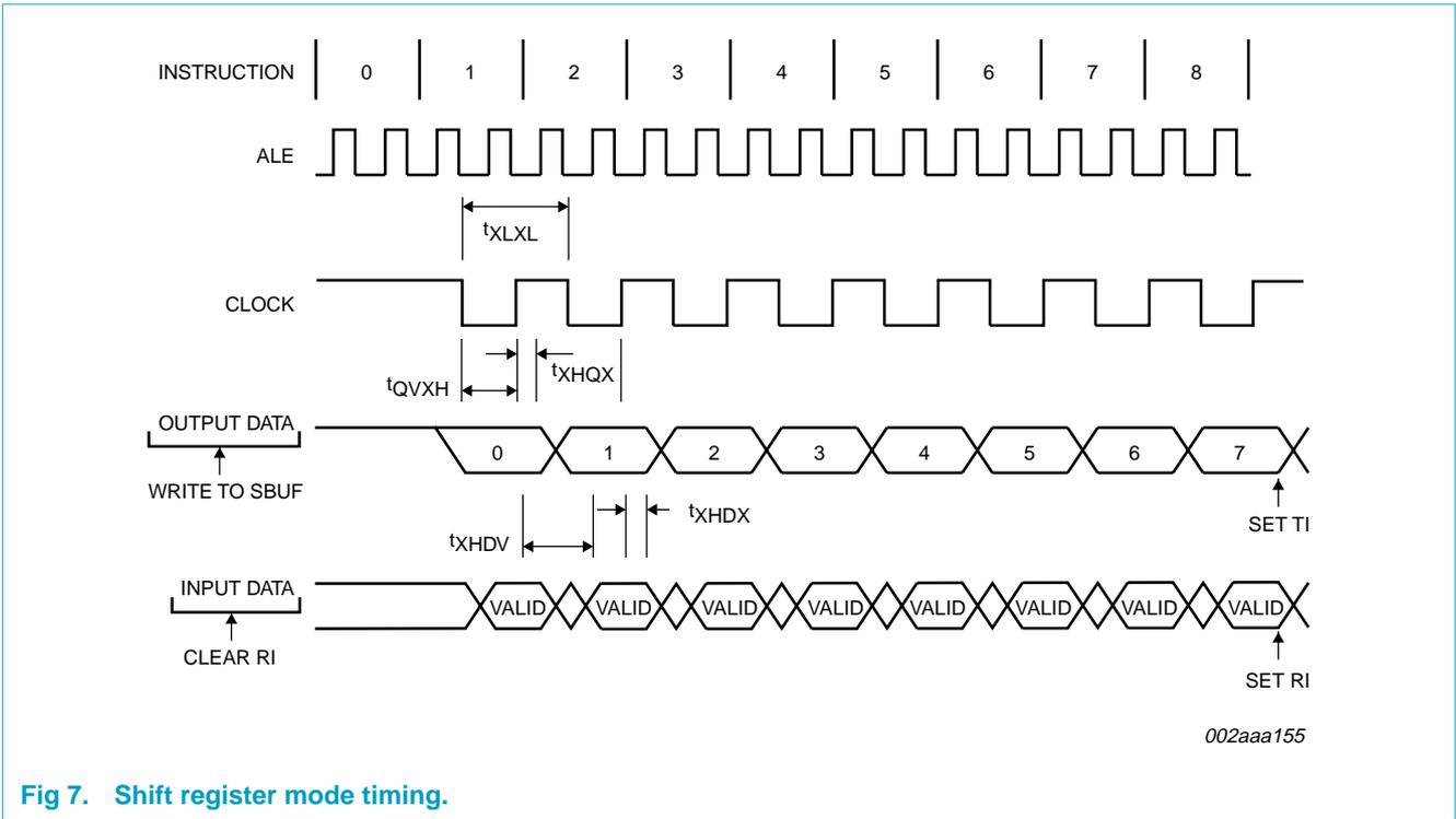
Fig 7. Shift register mode timing.
