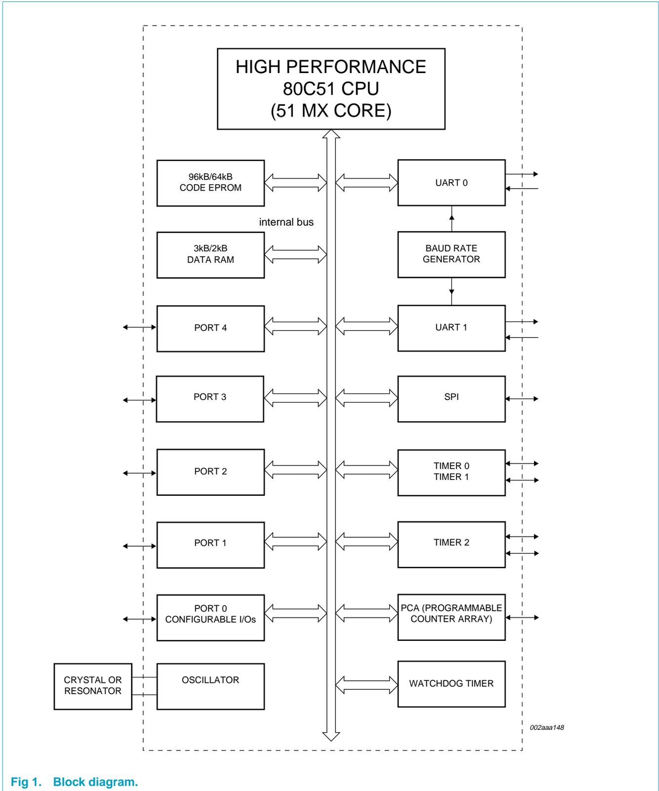
Fig 1. Block diagram.
