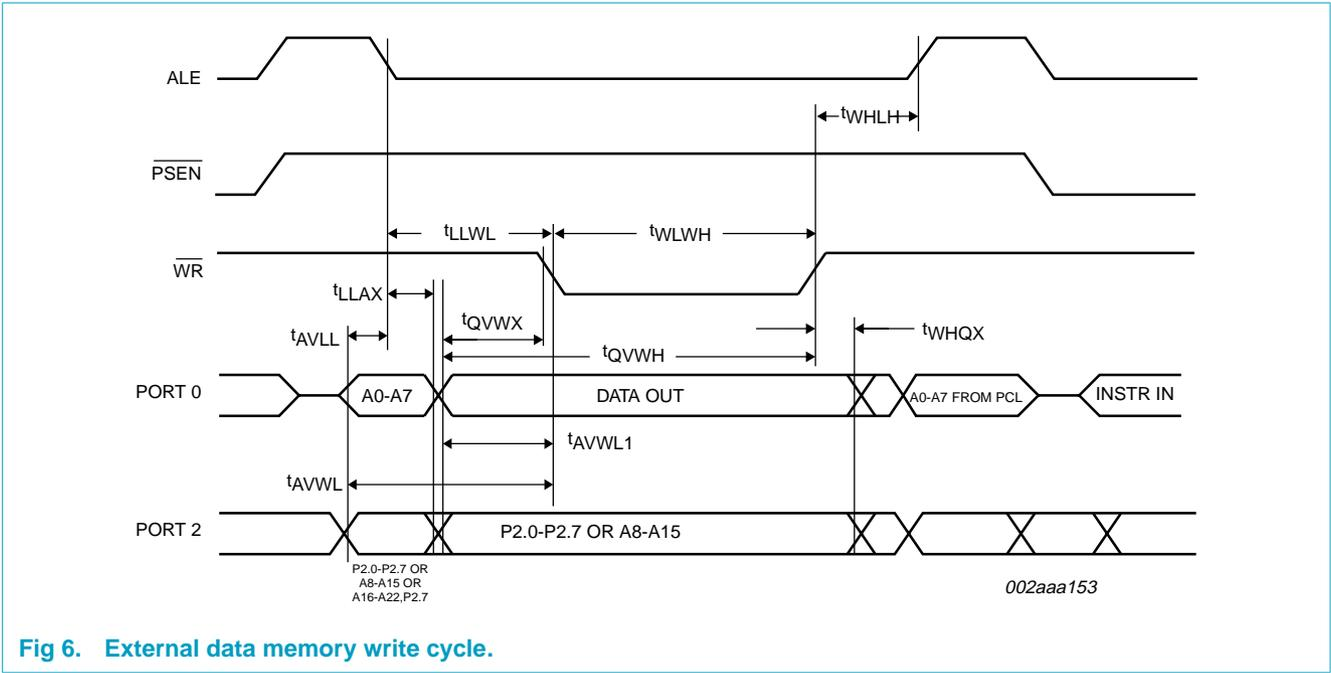
Fig 6. External data memory write cycle.
