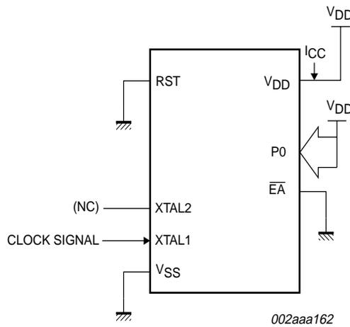
Fig 14. I<sub>CC</sub> test condition, idle mode (all other pins are disconnected).
