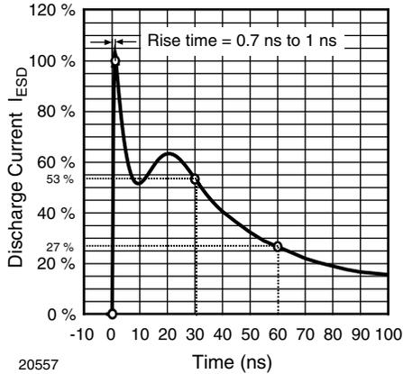
Fig. 1 - ESD Discharge Current Wave Form
