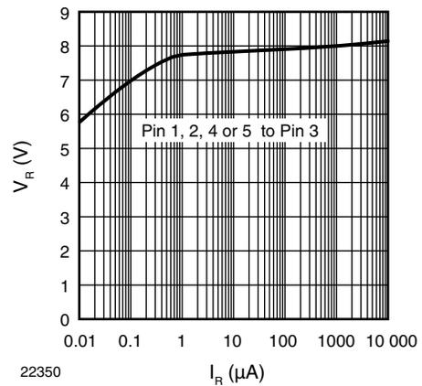
Fig. 5 - Typical Reverse Voltage  $V_R$  vs.
