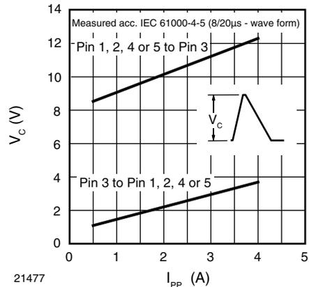
Fig. 6 - Typical Peak Clamping Voltage  $V_C$  vs.
