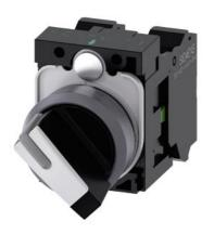
Selector switch, illuminable, 22 mm, round, plastic with metal front ring, white, selector switch, short, 2 switch positions O-I, latching, actuating angle  $90^\circ$ , 10:30h/13:30h, with holder, 1 NO, 1 NC, spring-type terminal, with laser labeling, upper case and lower case, always upper case at the beginning of the word
