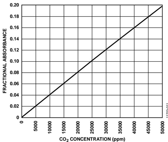
Figure 11. Fractional Absorbance vs. CO<sub>2</sub> Concentration for Typical [CN-0338](#) Board
