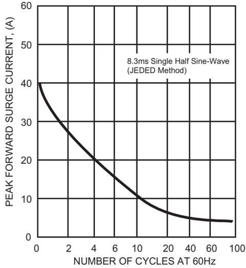
FIG. 2 - TYPICAL FORWARD CURRENT DERATING CURVE
