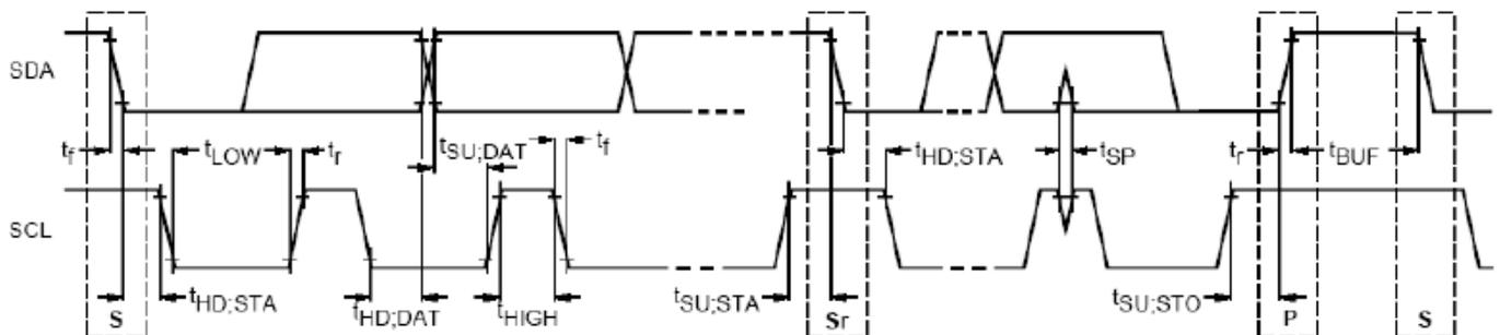
Definition of Timing for Full-Speed Mode Devices on the I<sup>2</sup>C Bus
