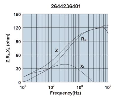
Impedance, reactance, and resistance vs. frequency.
