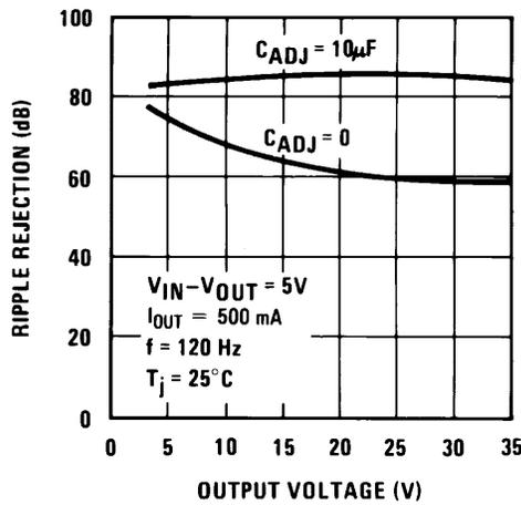
Figure 7-7. Ripple Rejection
