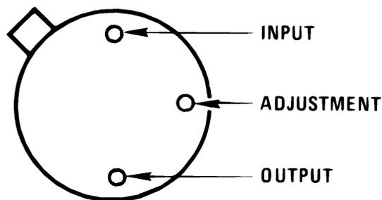
Figure 6-2. LM117H, LM117NDT NDT Package
