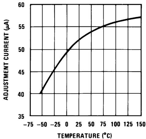
Figure 7-3. Adjustment Current
