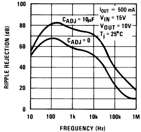
Figure 7-8. Ripple Rejection
