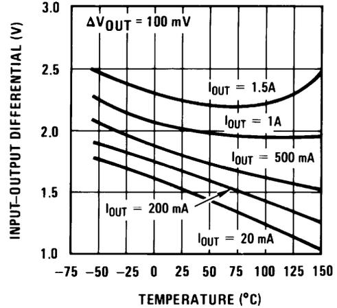
Figure 7-4. Dropout Voltage
