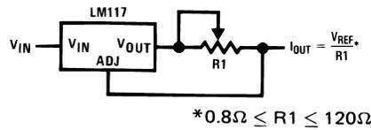
Figure 9-14. Precision Current Limiter
