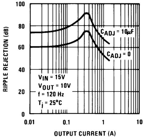
Figure 7-9. Ripple Rejection
