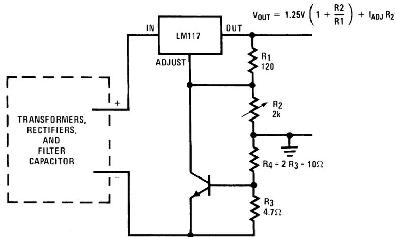
— Short circuit current is approximately  $\frac{600 \text{ mV}}{R_3}$ , or 120 mA
