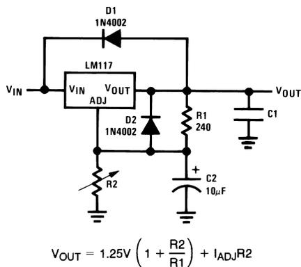
D1 protects against C1 (such as due to a  $V_{IN}$  short)
