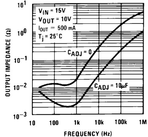
Figure 7-10. Output Impedance
