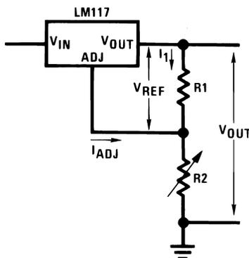
Since the 100- $\mu$ A current from the adjustment terminal represents an error term, the LM117 was designed to minimize  $I_{ADJ}$  and make it relatively constant with line and load changes. To do this, all quiescent operating current is returned to the output establishing a minimum load current requirement. If there is insufficient load on the output, the output will rise.
