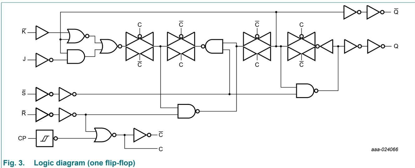
Fig. 3. Logic diagram (one flip-flop)
