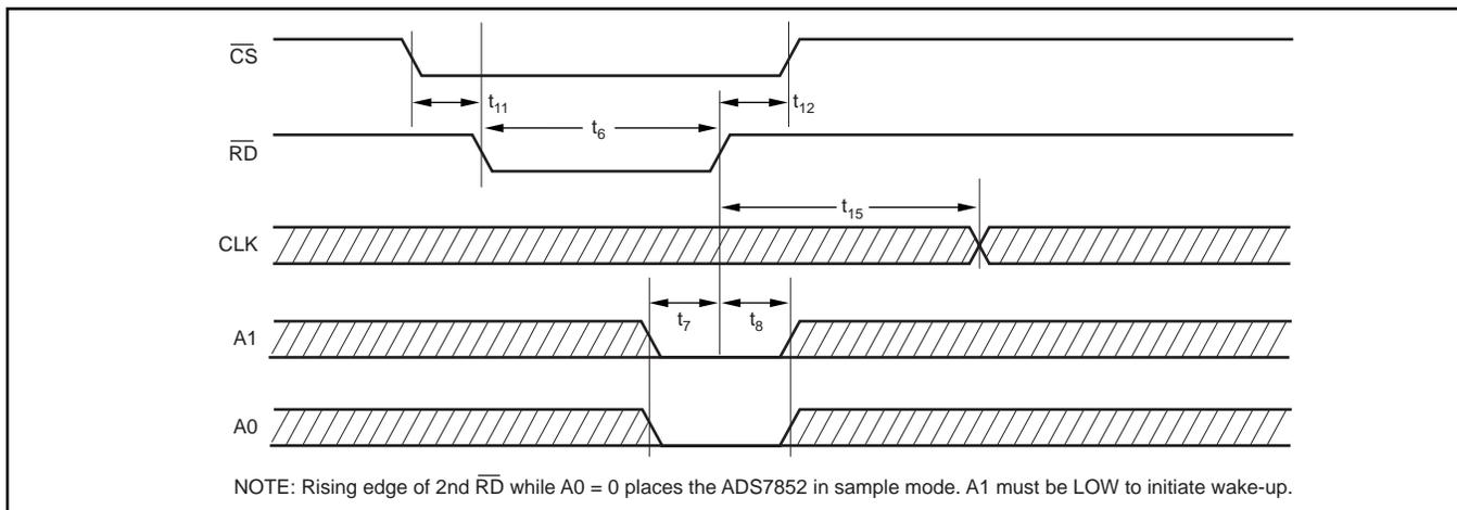
FIGURE 4. Initiating Wake-Up Using  $\overline{RD}$  and A0.
