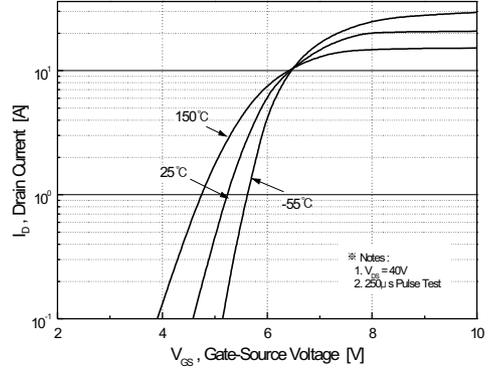
Figure 2. Transfer Characteristics
