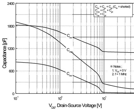
Figure 5. Capacitance Characteristics
