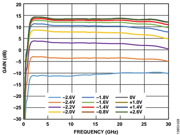
Figure 28. Gain vs. Frequency at Various  $V_{GG2}$  Voltages
