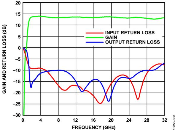
Figure 8. Response Gain and Return Loss vs. Frequency
