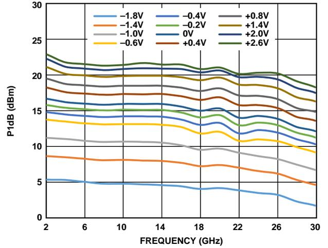
Figure 35. P1dB vs. Frequency at Various  $V_{GG2}$  Voltages
