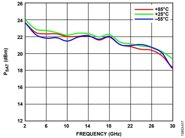
Figure 17. P<sub>SAT</sub> vs. Frequency at Various Temperatures
