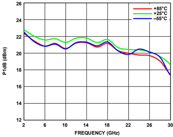
Figure 14. P1dB vs. Frequency at Various Temperatures
