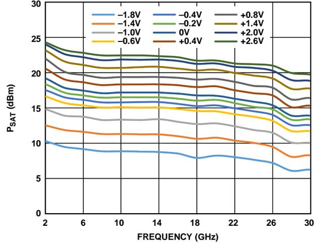
Figure 36.  $P_{SAT}$  vs. Frequency at Various  $V_{GG2}$  Voltages
