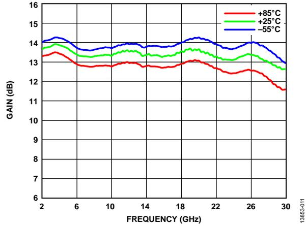
Figure 11. Gain vs. Frequency at Various Temperatures
