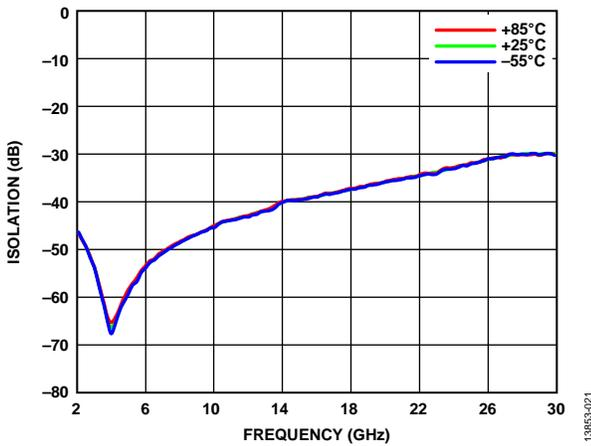
Figure 21. Reverse Isolation vs. Frequency at Various Temperatures
