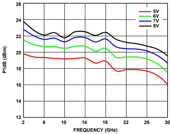
Figure 15. P1dB vs. Frequency at Various Supply Voltages
