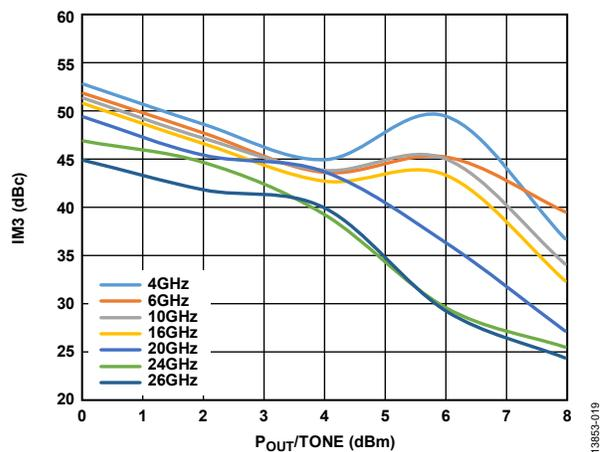
Figure 19. Output Third Order Intermodulation (IM3) vs. P<sub>OUT</sub>/Tone for Various Frequencies at V<sub>DD</sub> = 6 V
