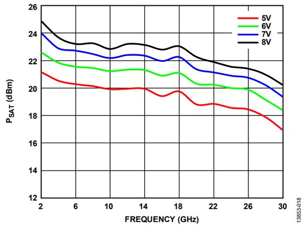
Figure 18. P<sub>SAT</sub> vs. Frequency at Various Supply Voltages
