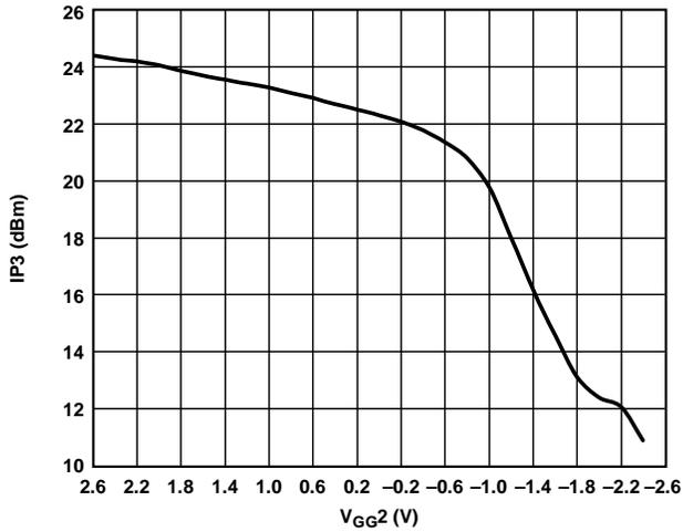
Figure 33. Output IP3 vs.  $V_{GG2}$  at 16 GHz
