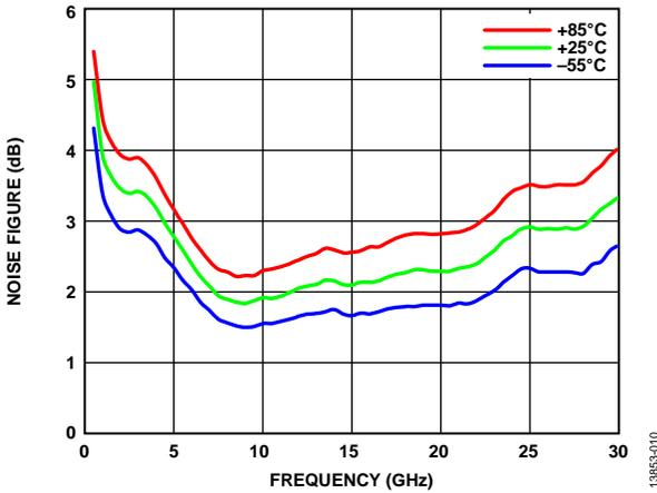
Figure 10. Noise Figure vs. Frequency at Various Temperatures
