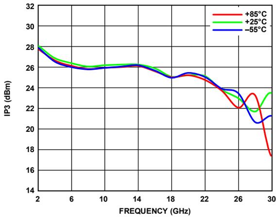
Figure 16. Output IP3 vs. Frequency for Various Temperatures at P<sub>OUT</sub> = 0 dBm/Tone
