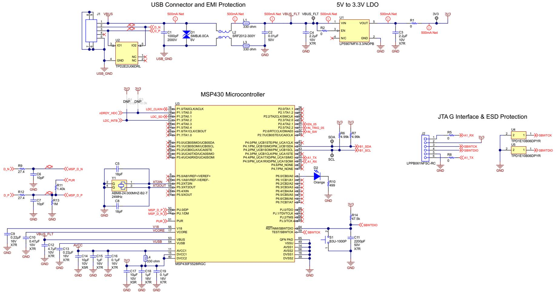
Figure 88. Touch on Metal Buttons With Integrated Haptic Feedback Schematic—Page 1
