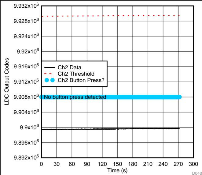
Figure 77. LDC Ch2 Data During Surge (+0.5 kV, From VBUS to GND) Test—Big Button Channel
