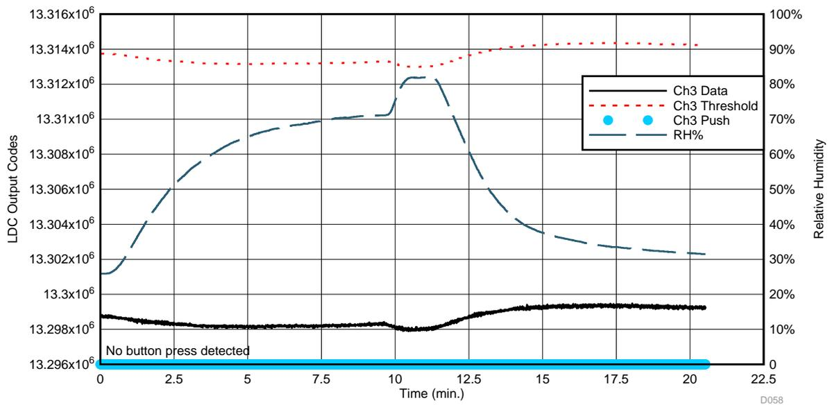
Figure 53. LDC Ch3 Data During Relative Humidity “Shock” Test—Little Button Channel
