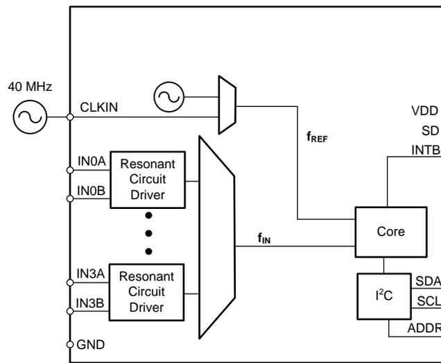
**Figure 5. LDC1614 Functional Block Diagram**
