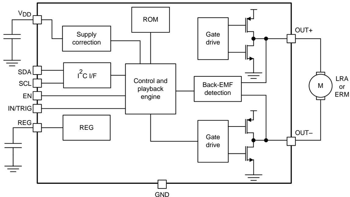
Figure 6. DRV2605L Functional Block Diagram
