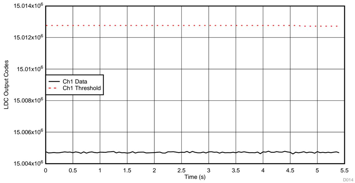
Figure 36. LDC Ch1 Data During LRA Activation—Up Button Channel
