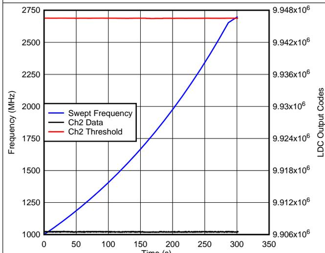
**Figure 71. LDC Ch2 Data During Radiated Immunity (1 GHz – 2.7 GHz, Vertical Polarization) Test—Big Button Channel**
