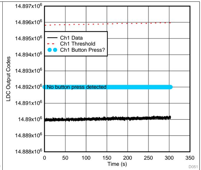
Figure 80. LDC Ch1 Data During Surge (-0.5 kV, From VBUS to GND) Test—Up Button Channel
