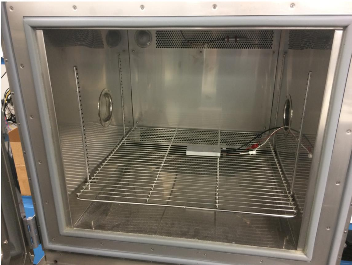
**Figure 43. Temperature and Relative Humidity Test Setup**
