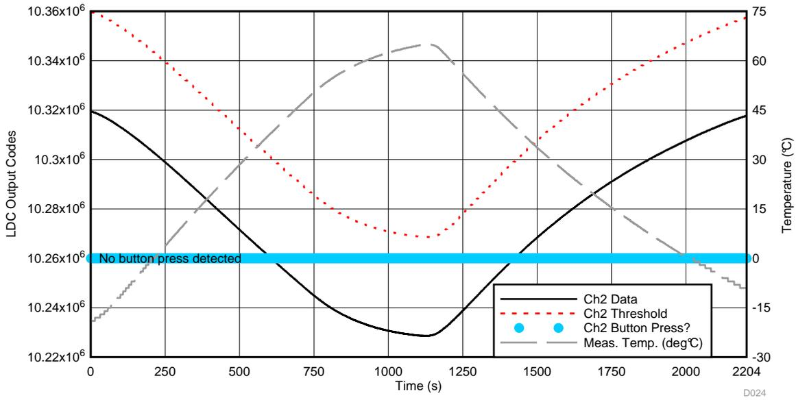
Figure 47. LDC Ch2 Data During Thermal “Shock” Test—*Big* Button Channel
