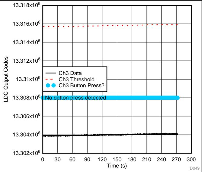
Figure 78. LDC Ch3 Data During Surge (+0.5 kV, From VBUS to GND) Test—Little Button Channel
