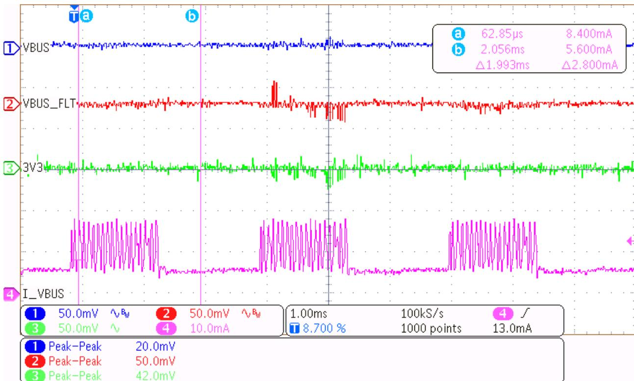
**Figure 39. Power Data During LDC Measurement**
