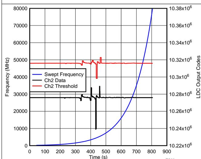
Figure 86. LDC Ch2 Data During Conducted Immunity Test—Big Button Channel
