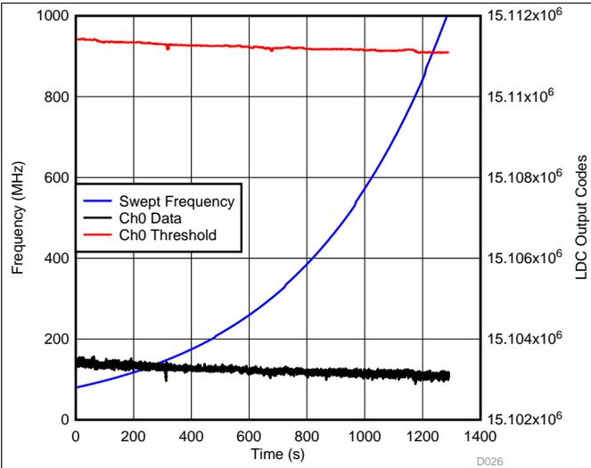
**Figure 57. LDC Ch0 Data During Radiated Immunity (80 MHz – 1 GHz, Horizontal Polarization) Test—Down Button Channel**
