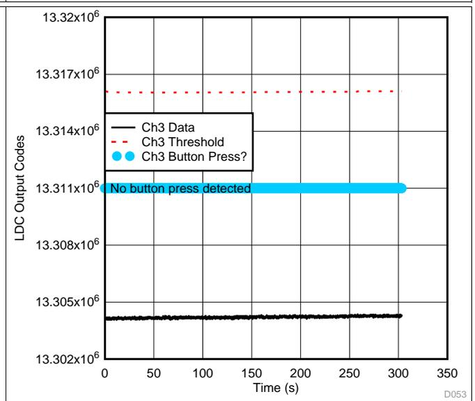
Figure 82. LDC Ch3 Data During Surge (-0.5 kV, From VBUS to GND) Test—Little Button Channel
