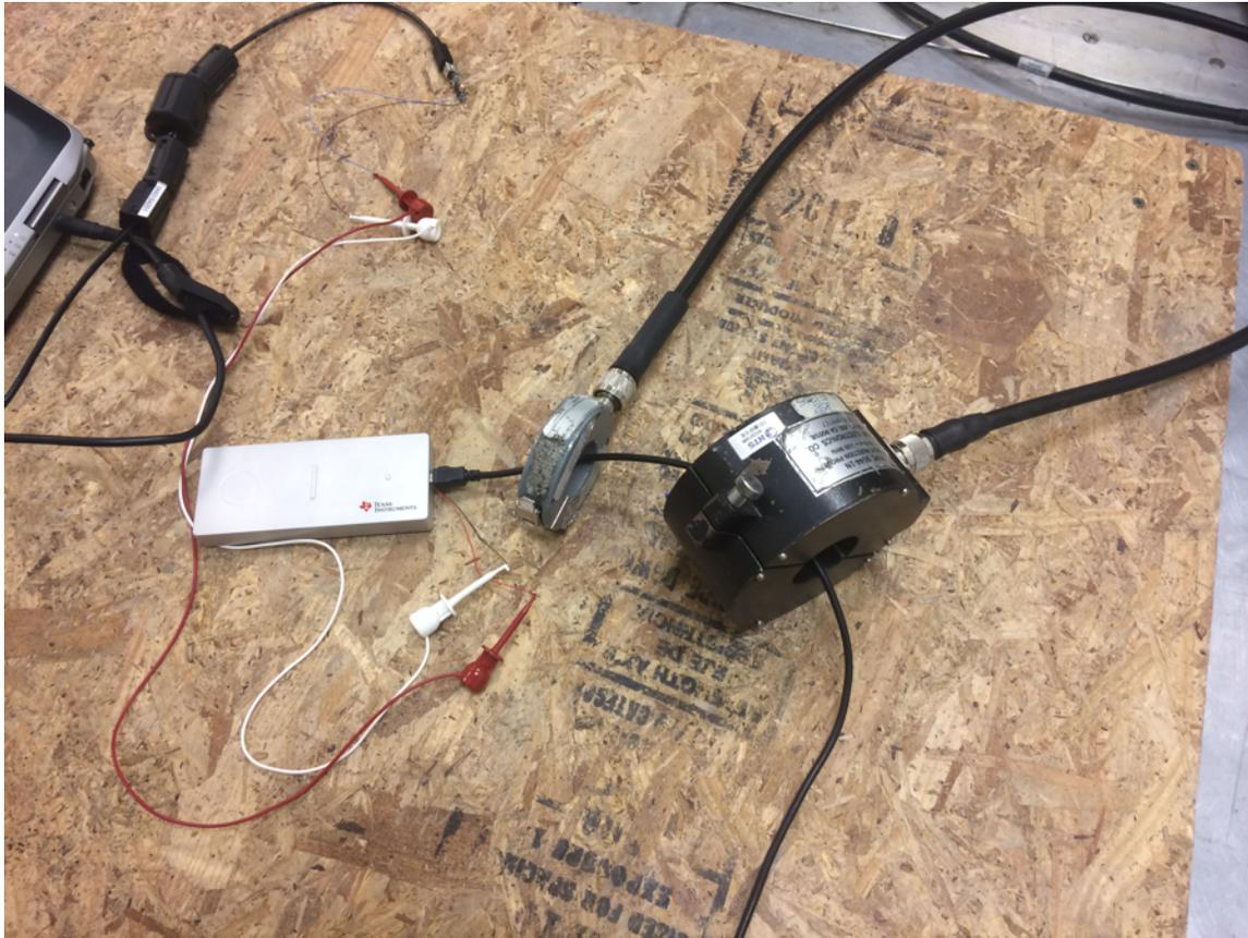
**Figure 83. IEC 61000-4-6 Conducted Immunity Test Setup**
