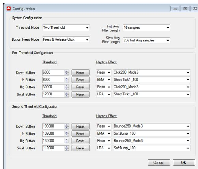
**Figure 17. Firmware Configuration**
