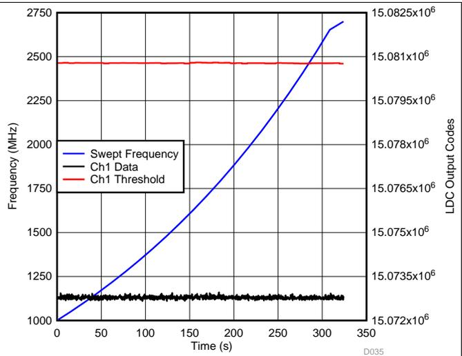
**Figure 66. LDC Ch1 Data During Radiated Immunity (1 GHz – 2.7 GHz, Horizontal Polarization) Test—Up Button Channel**
