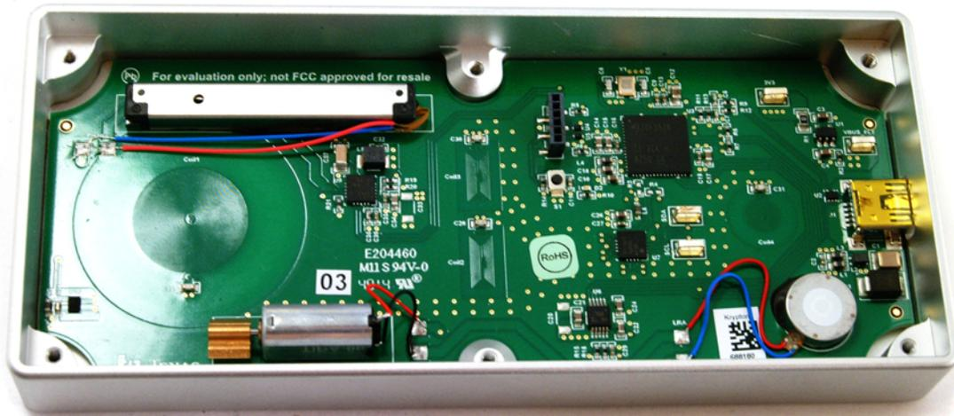
**Figure 14. Touch on Metal Buttons With Integrated Haptic Feedback Reference Design Hardware**
