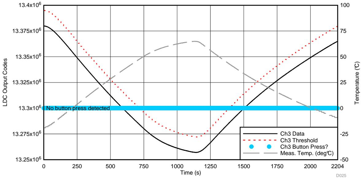
Figure 48. LDC Ch3 Data During Thermal “Shock” Test—*Little* Button Channel
