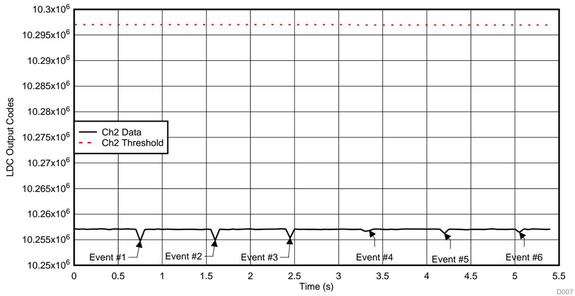
Figure 29. LDC Ch2 Data During Piezo Activation—*Big Button Channel*
