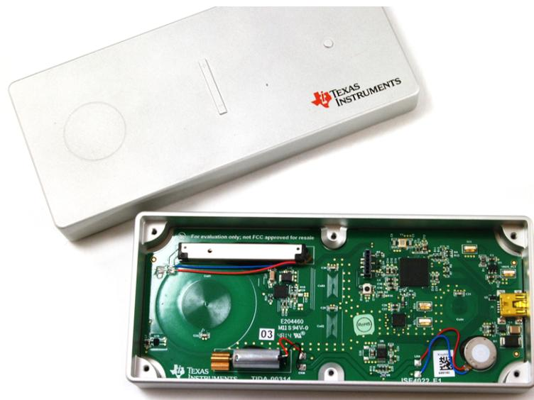
**Figure 2. Touch on Metal Buttons With Integrated Haptic Feedback Mechanical Enclosure Detail**
