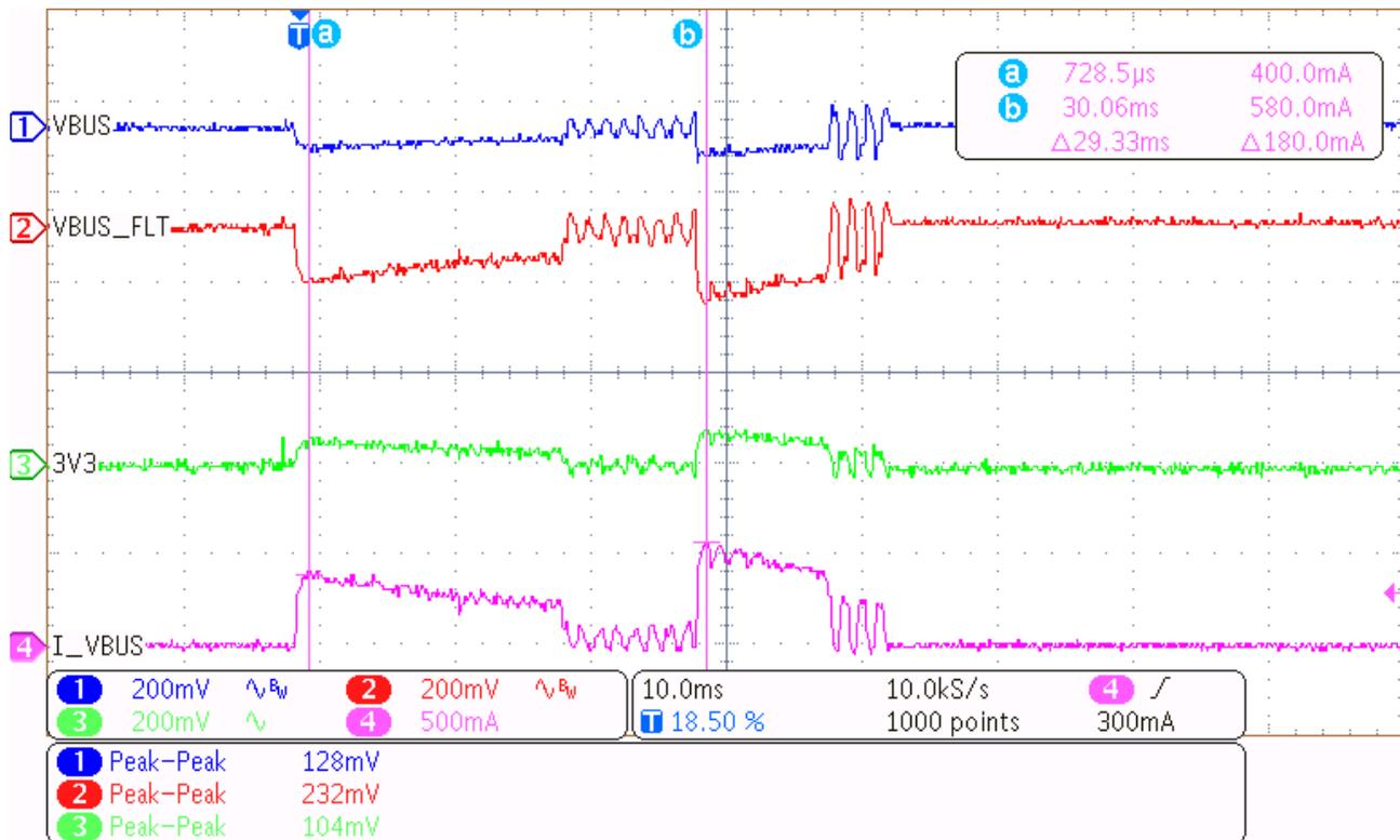
Figure 41. Power Data During ERM Actuator Operation
