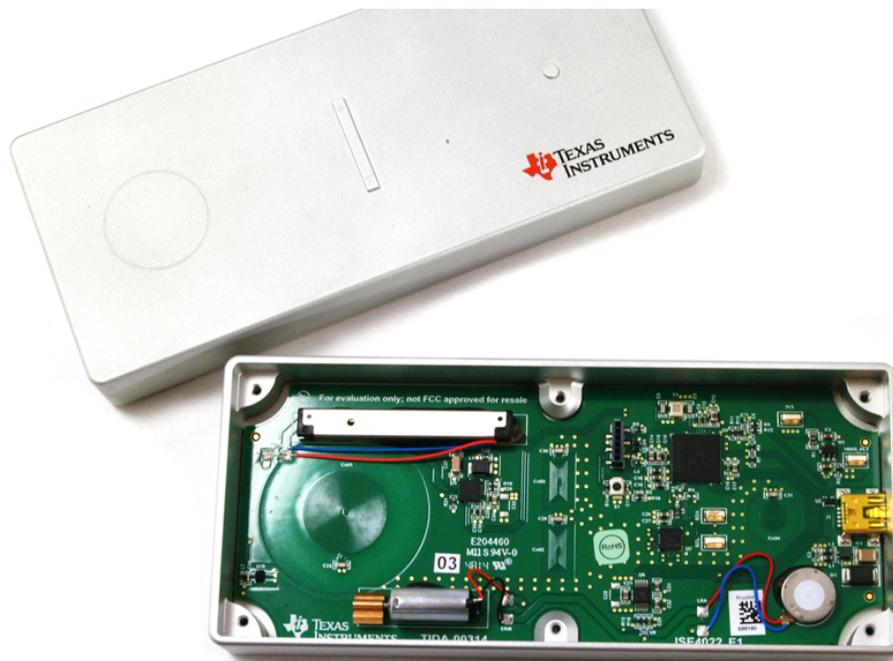
**Figure 15. Touch on Metal Buttons With Integrated Haptic Feedback Reference Design Hardware**
