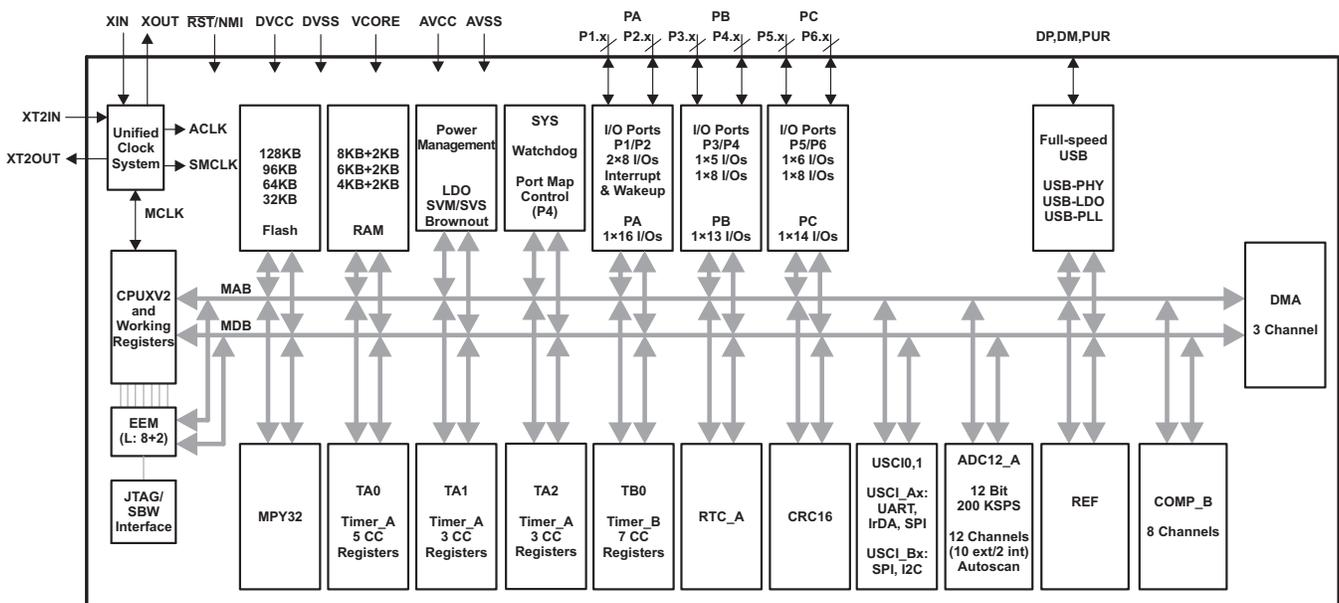
**Figure 9. MSP430F5528 Functional Block Diagram**
