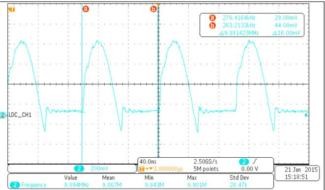
**Figure 24. LC Tank Baseline Resonant Frequency—Ch1 (Up Button)**
