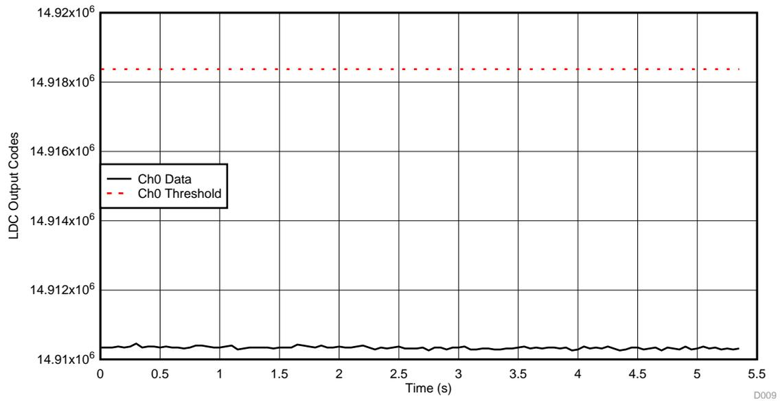
**Figure 31. LDC Ch0 Data During ERM Activation—Down Button Channel**
