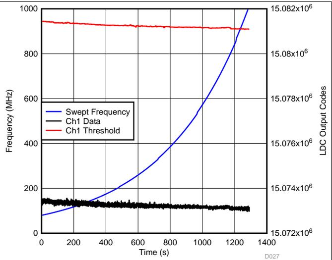
**Figure 58. LDC Ch1 Data During Radiated Immunity (80 MHz – 1 GHz, Horizontal Polarization) Test—Up Button Channel**
