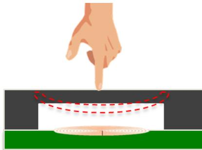
**Figure 1. Mechanical Deflection Detail**
