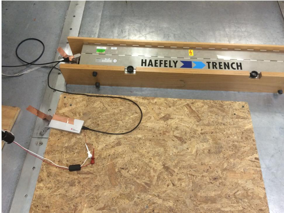
**Figure 73. IEC 61000-4-4 EFT Test Setup**
