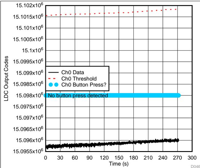
Figure 75. LDC Ch0 Data During Surge (+0.5 kV, From VBUS to GND) Test—Down Button Channel
