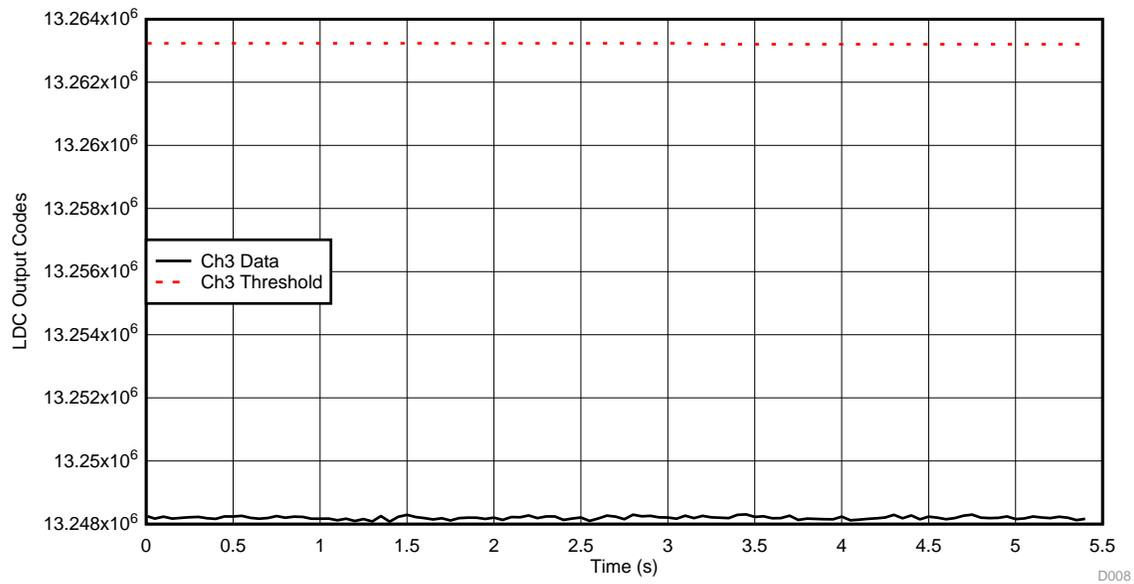
Figure 30. LDC Ch3 Data During Piezo Activation—*Little Button Channel*
