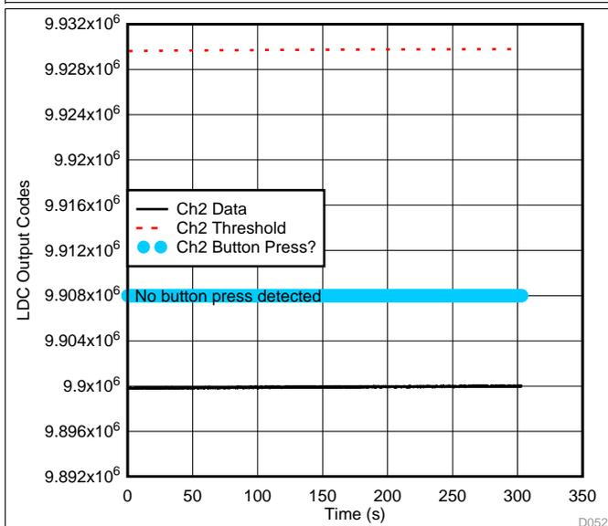
Figure 81. LDC Ch2 Data During Surge (-0.5 kV, From VBUS to GND) Test—Big Button Channel
