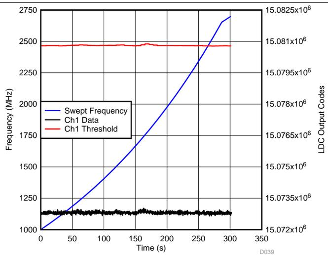
**Figure 70. LDC Ch1 Data During Radiated Immunity (1 GHz – 2.7 GHz, Vertical Polarization) Test—Up Button Channel**
