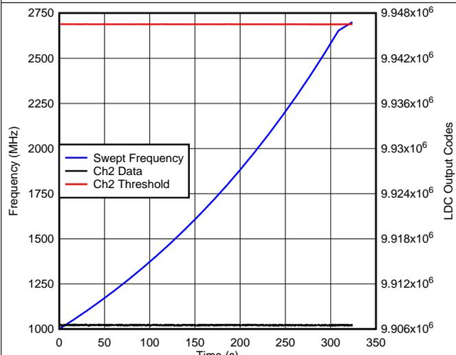
**Figure 67. LDC Ch2 Data During Radiated Immunity (1 GHz – 2.7 GHz, Horizontal Polarization) Test—Big Button Channel**
