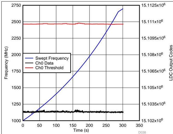
**Figure 69. LDC Ch0 Data During Radiated Immunity (1 GHz – 2.7 GHz, Vertical Polarization) Test—Down Button Channel**
