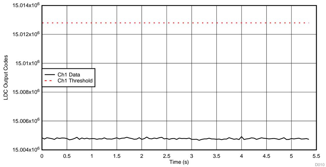
**Figure 32. LDC Ch1 Data During ERM Activation—Up Button Channel**
