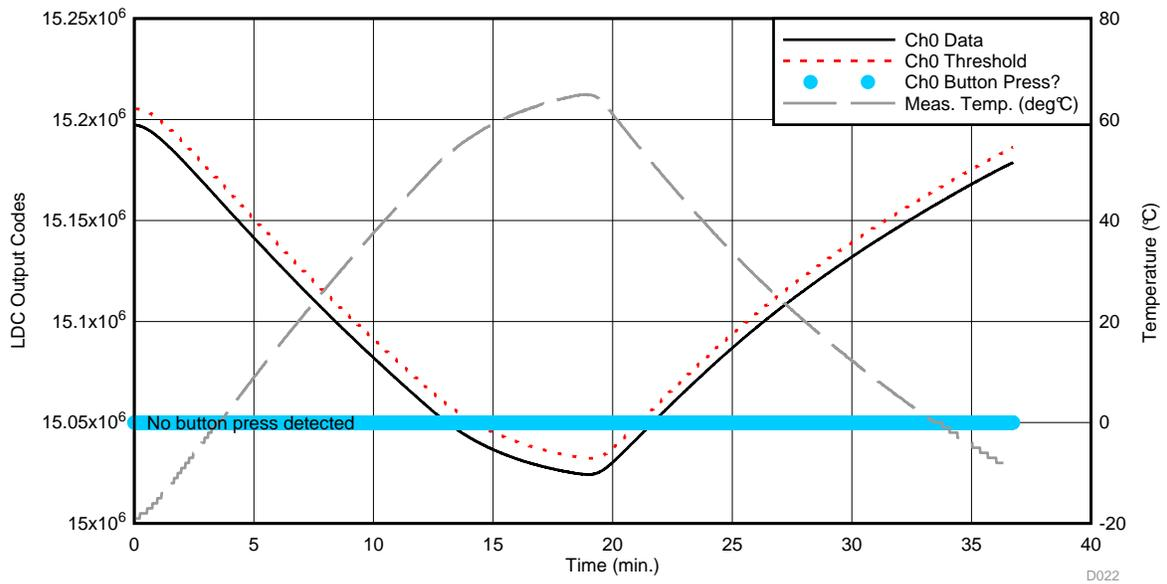
Figure 45. LDC Ch0 Data During Thermal “Shock” Test—Down Button Channel
