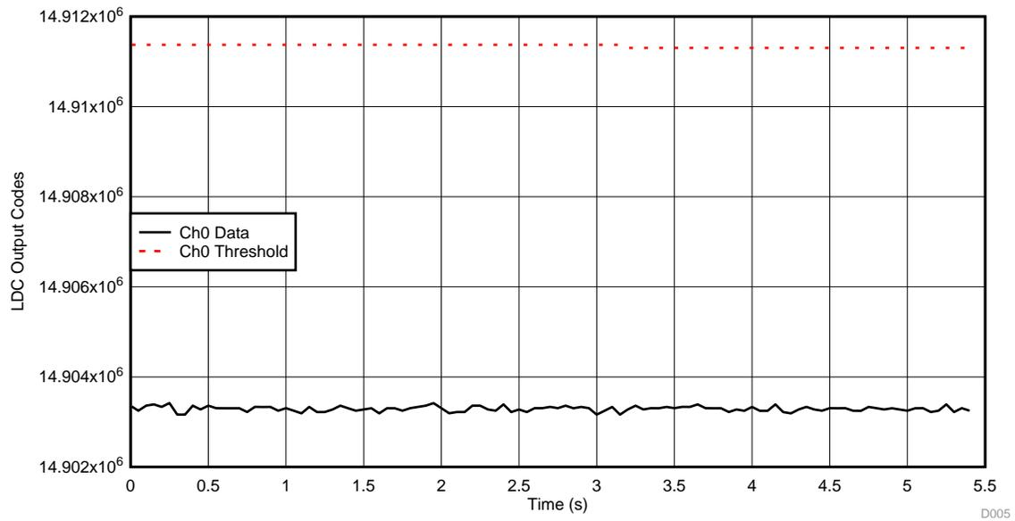
**Figure 27. LDC Ch0 Data During Piezo Activation—Down Button Channel**
