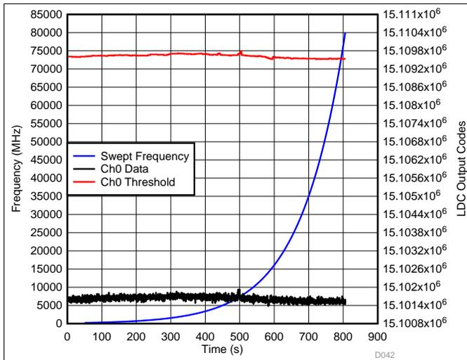
Figure 84. LDC Ch0 Data During Conducted Immunity Test—Down Button Channel
