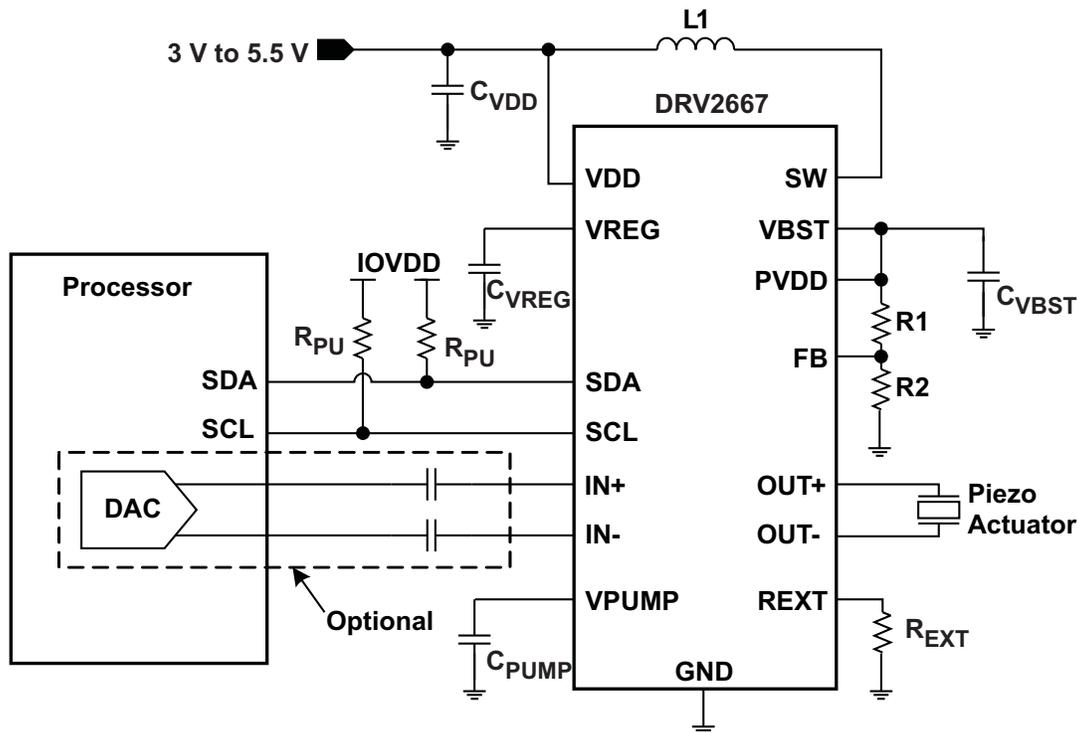
Figure 7. DRV2667 System Diagram
