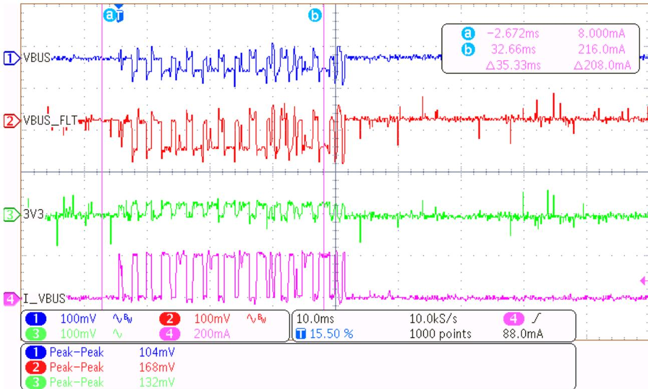
Figure 42. Power Data During LRA Actuator Operation
