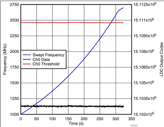
**Figure 65. LDC Ch0 Data During Radiated Immunity (1 GHz – 2.7 GHz, Horizontal Polarization) Test—Down Button Channel**
