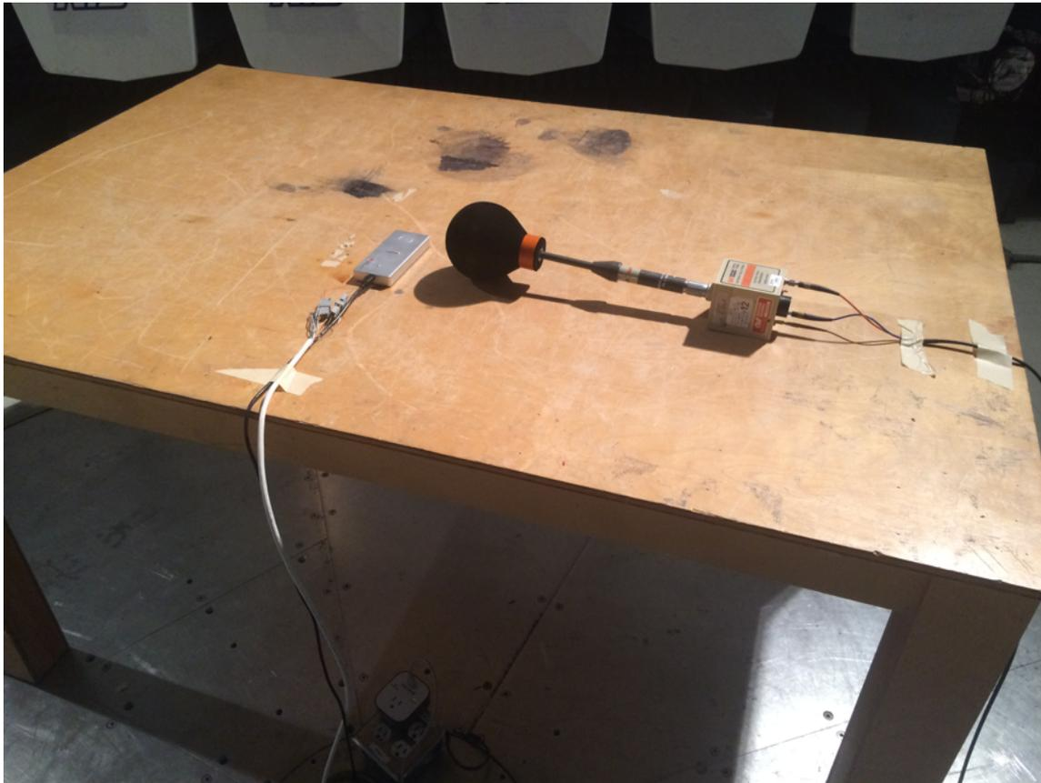
**Figure 56. IEC 61000-4-3 Radiated Immunity Test Setup**
