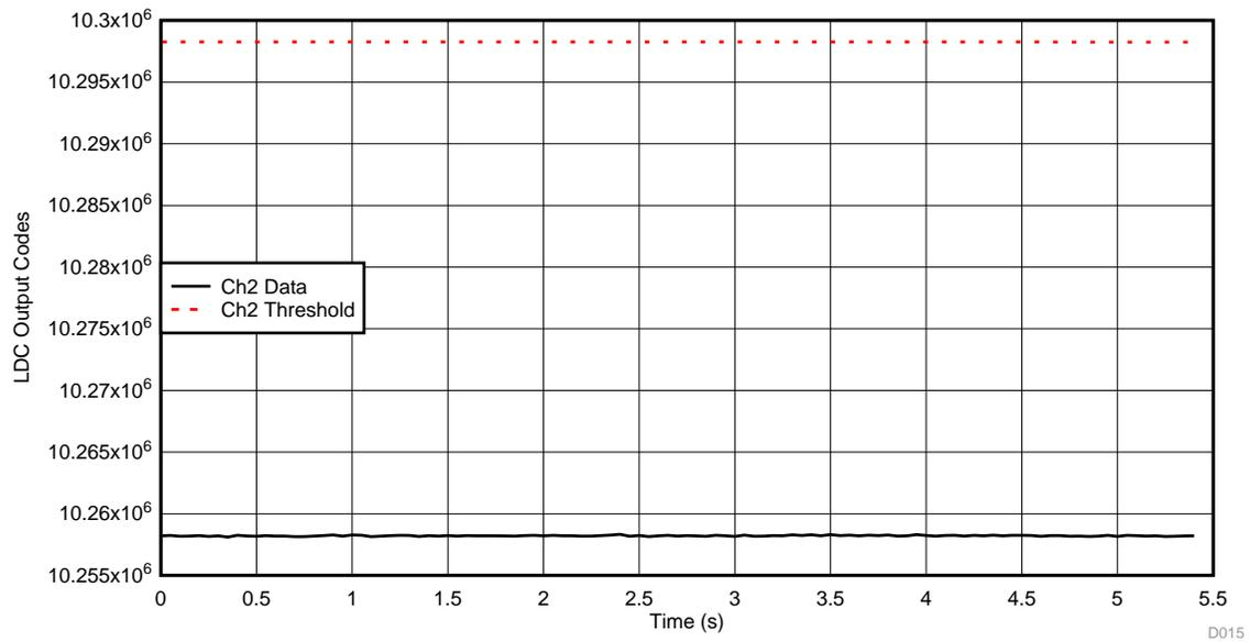
Figure 37. LDC Ch2 Data During LRA Activation—*Big* Button Channel
