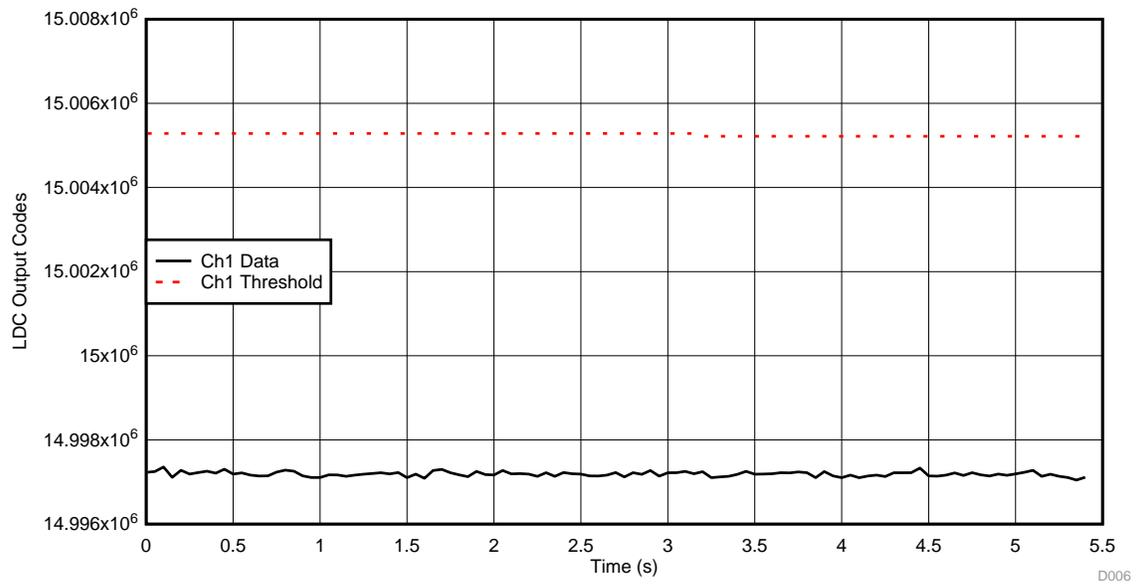
**Figure 28. LDC Ch1 Data During Piezo Activation—Up Button Channel**
