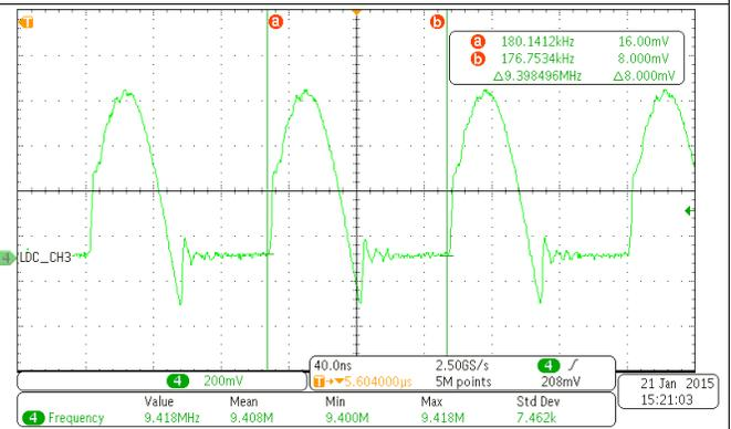
**Figure 26. LC Tank Baseline Resonant Frequency—Ch3 (Little Button)**
