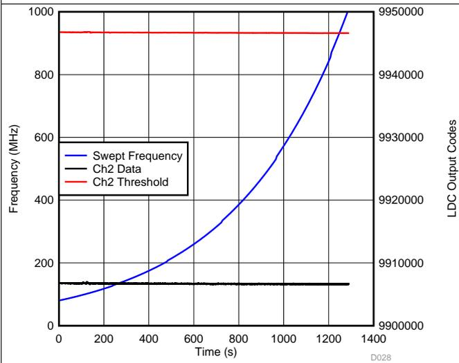
**Figure 59. LDC Ch2 Data During Radiated Immunity (80 MHz – 1 GHz, Horizontal Polarization) Test—Big Button Channel**
