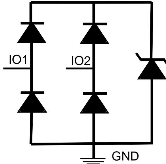
Figure 12. TPD2E2U06 Functional Block Diagram
