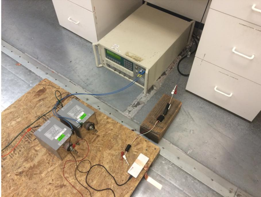
**Figure 74. IEC 61000-4-5 Surge Test Setup**
