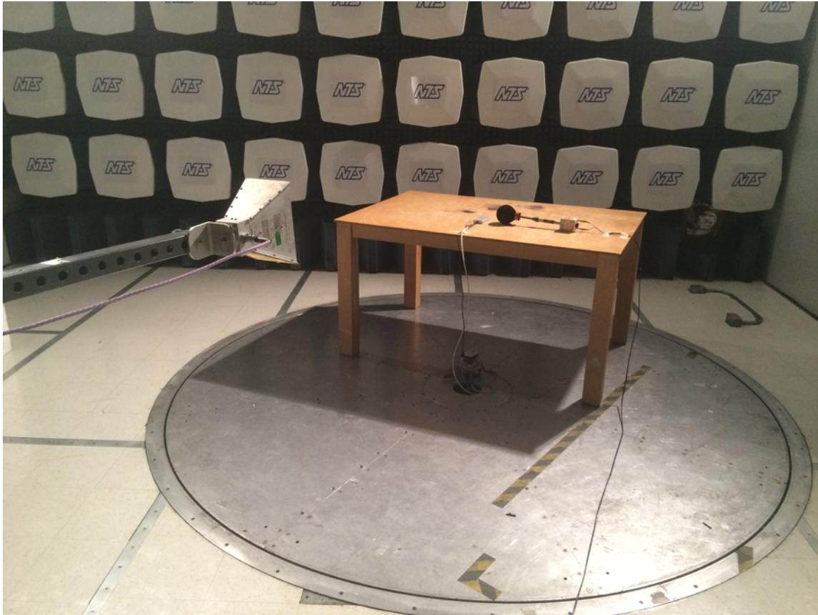
**Figure 55. IEC 61000-4-3 Radiated Immunity Test Setup**
