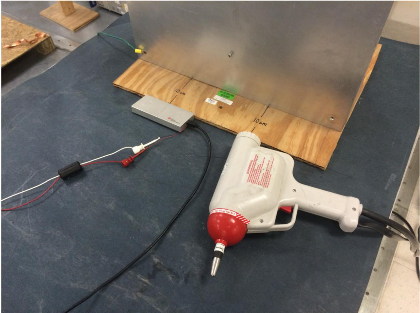
**Figure 54. IEC 61000-4-2 ESD Test Setup**
