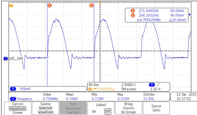
**Figure 23. LC Tank Baseline Resonant Frequency—Ch0 (Down Button)**
