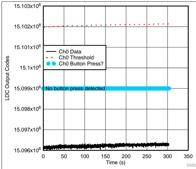
Figure 79. LDC Ch0 Data During Surge (-0.5 kV, From VBUS to GND) Test—Down Button Channel
