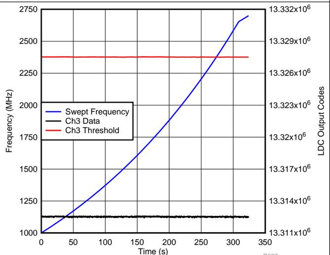
**Figure 68. LDC Ch3 Data During Radiated Immunity (1 GHz – 2.7 GHz, Horizontal Polarization) Test—Little Button Channel**
