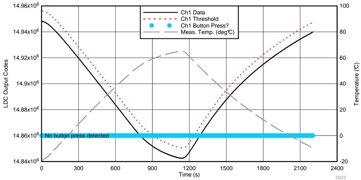
Figure 46. LDC Ch1 Data During Thermal “Shock” Test—Up Button Channel
