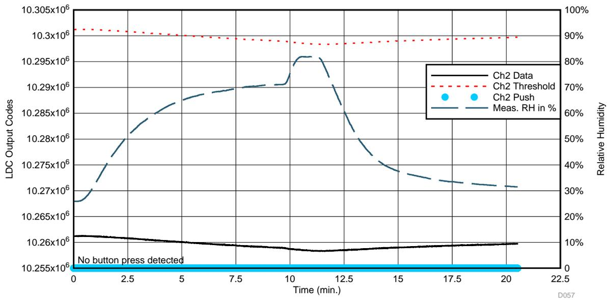
Figure 52. LDC Ch2 Data During Relative Humidity “Shock” Test—Big Button Channel
