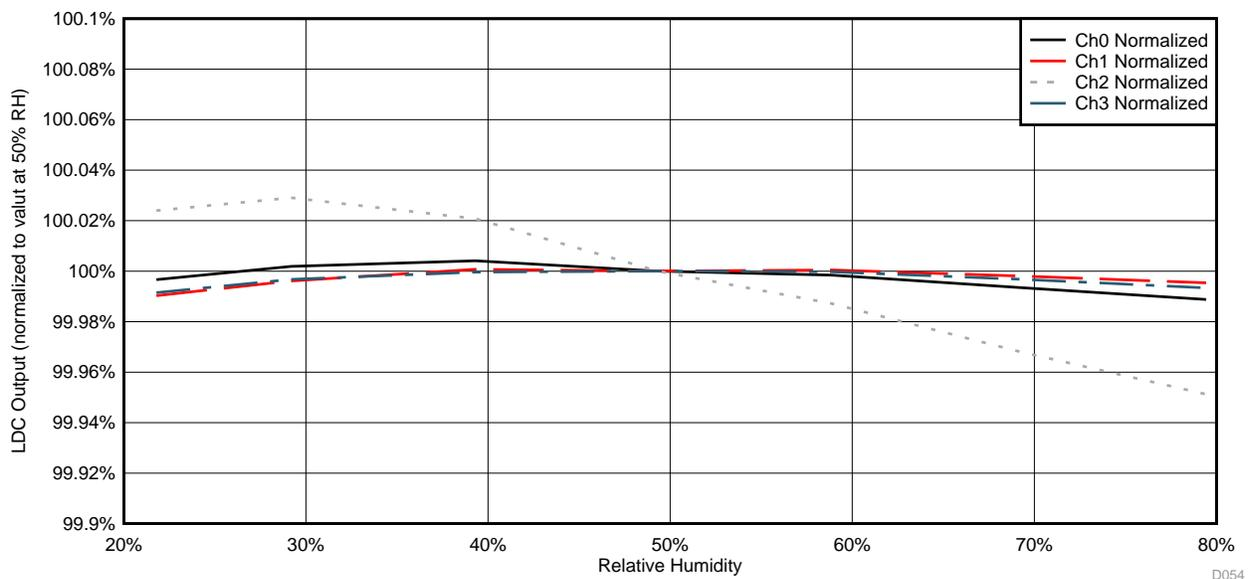
**Figure 49. LDC1614 Data Over Relative Humidity—All Channels**
