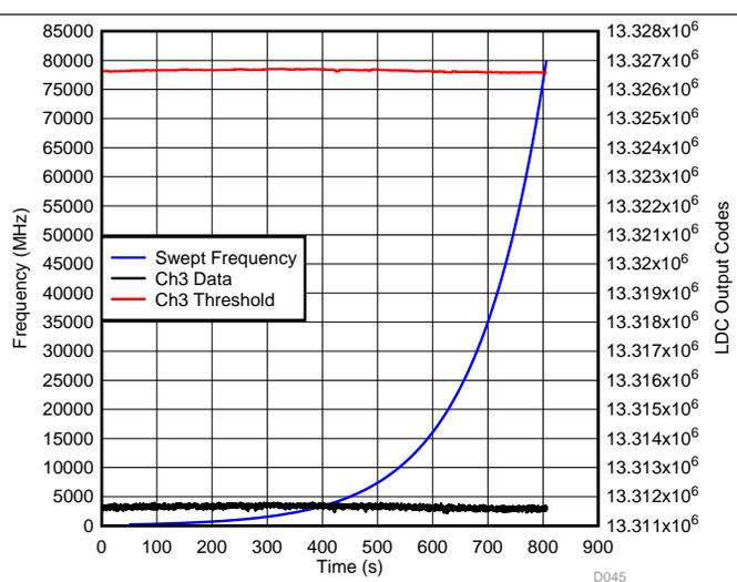
Figure 87. LDC Ch3 Data During Conducted Immunity Test—Little Button Channel
