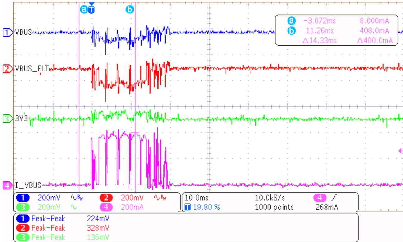
Figure 40. Power Data During Piezo Actuator Operation
