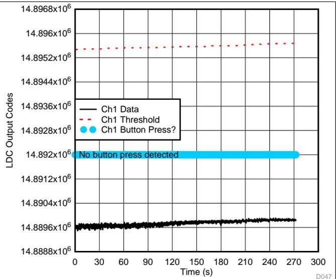
Figure 76. LDC Ch1 Data During Surge (+0.5 kV, From VBUS to GND) Test—Up Button Channel
