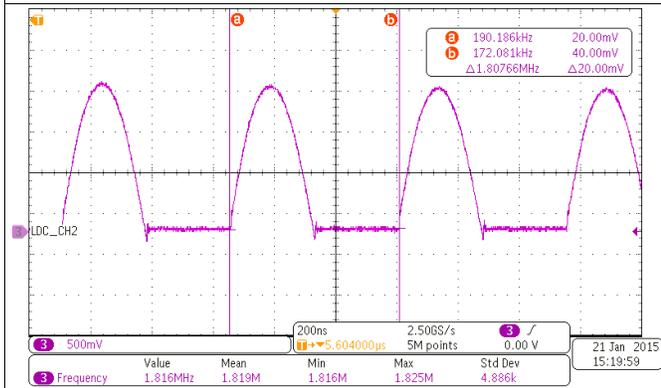
**Figure 25. LC Tank Baseline Resonant Frequency—Ch2 (Big Button)**
