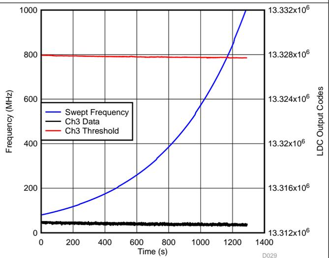
**Figure 60. LDC Ch3 Data During Radiated Immunity (80 MHz – 1 GHz, Horizontal Polarization) Test—Little Button Channel**
