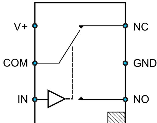
Figure 11. TS5A12301E Logic Diagram
