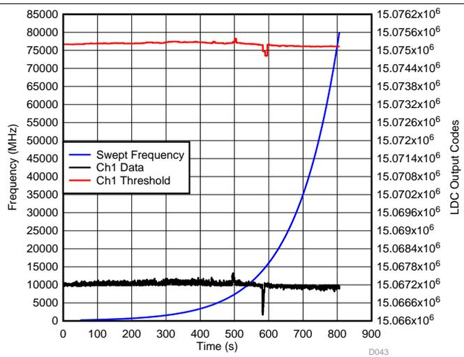
Figure 85. LDC Ch1 Data During Conducted Immunity Test—Up Button Channel
