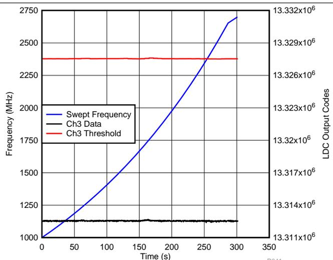
**Figure 72. LDC Ch3 Data During Radiated Immunity (1 GHz – 2.7 GHz, Vertical Polarization) Test—Little Button Channel**
