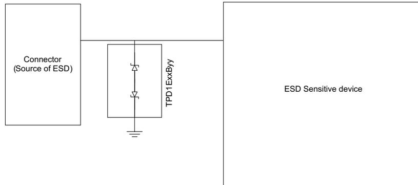
**Figure 13. TPD1E10B06 Device Configuration**
