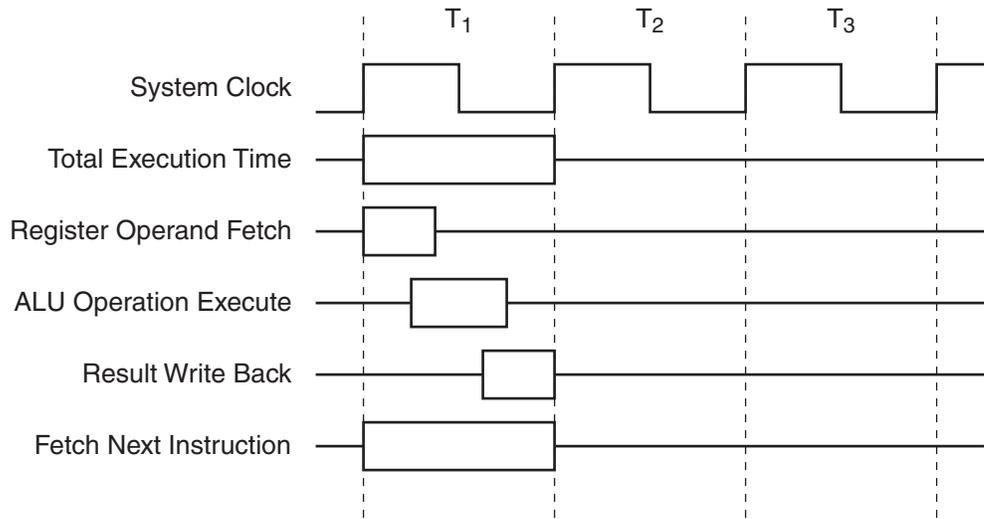
**Figure 8-3.** Two-Cycle ALU Operation (Example: ADD A, #data)
