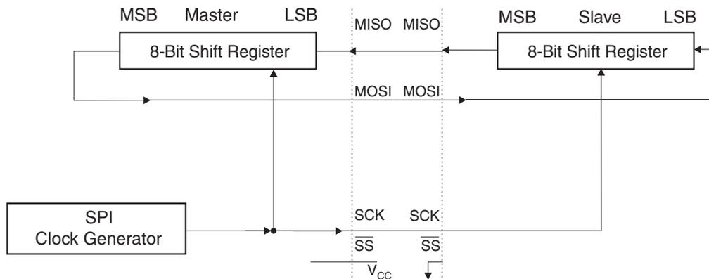
**Figure 19-2.** SPI Block Diagram
