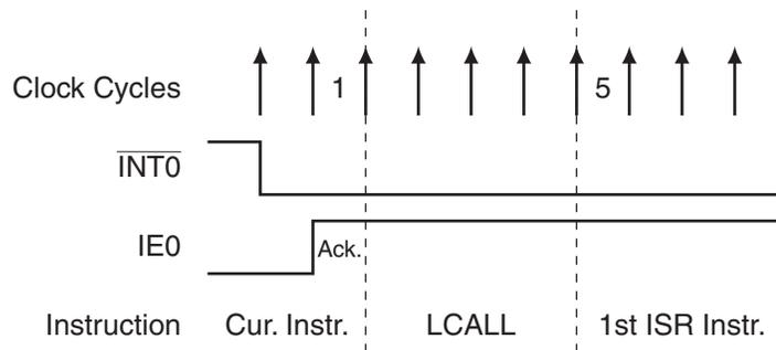
**Figure 14-2.** Maximum Interrupt Response Time
