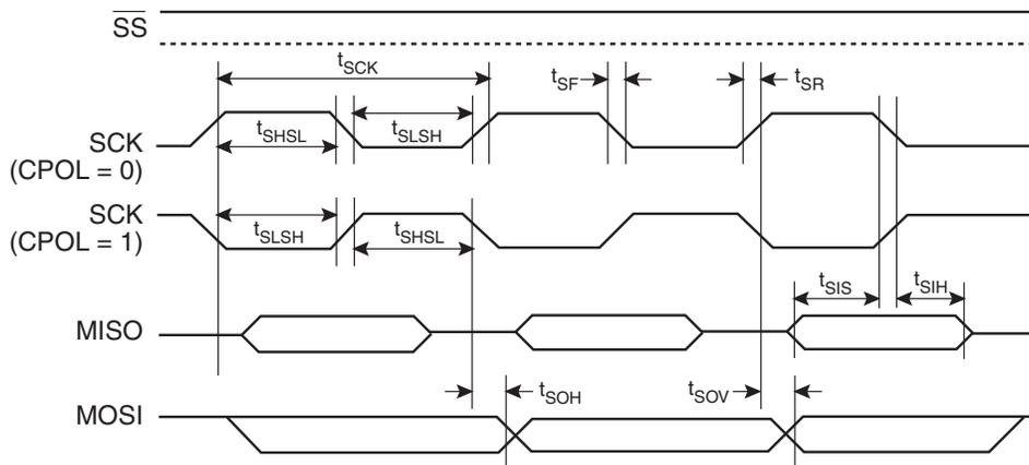
**Figure 24-4.** SPI Slave Timing (CPHA = 1)
