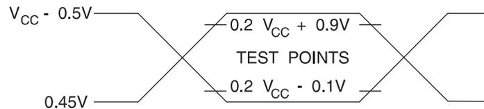
Note: 1. AC Inputs during testing are driven at  $V_{CC} - 0.5\text{V}$  for a logic "1" and  $0.45\text{V}$  for a logic "0". Timing measurements are made at  $V_{IH\text{ min.}}$  for a logic "1" and  $V_{IL\text{ max.}}$  for a logic "0".
