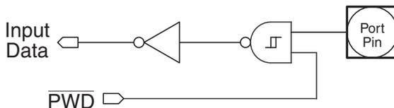
Figure 15-3. Input Only for P3.2 and P3.3
