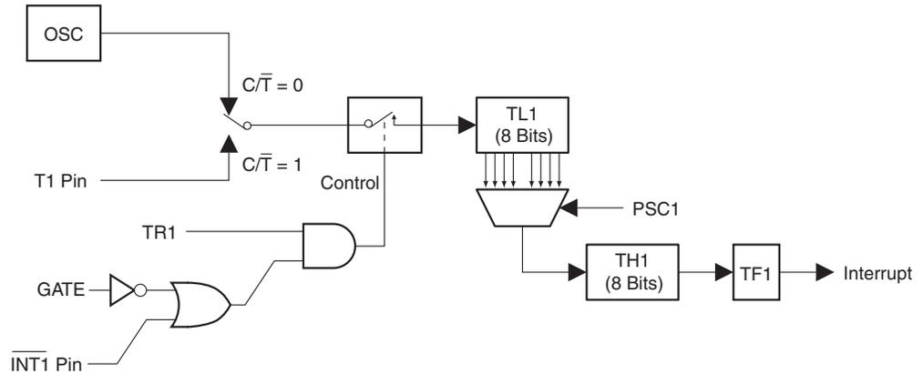
Mode 0 operation is the same for Timer 0 as for Timer 1, except that TR0, TF0 and  $\overline{\text{INT0}}$  replace the corresponding Timer 1 signals in Figure 16-1. There are two different GATE bits, one for Timer 1 (TMOD.7) and one for Timer 0 (TMOD.3).
