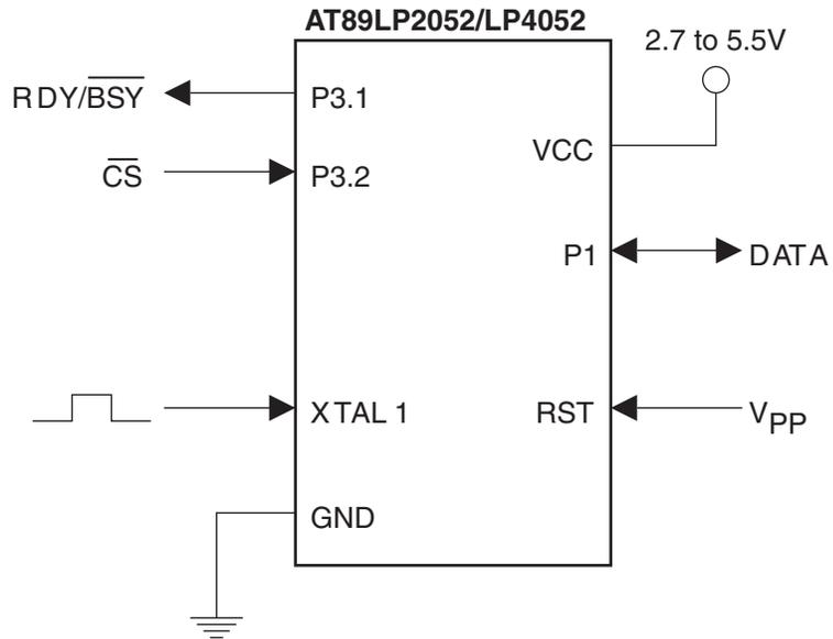
Note: Sampling of pin P3.1 ( $\overline{RDY/BSY}$ ) is optional. During Parallel Programming, P3.1 will be pulled low while the device is busy. Note that it does not require an external passive pull-up to  $V_{CC}$ .
