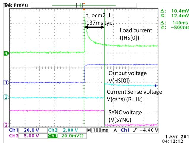
**Figure 15. Current sense blanking during overcurrent window activity**
