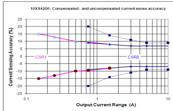
Figure 20. Current sense accuracy versus output current
