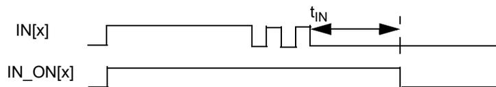
Figure 11. Relation between signals  $IN(x)$  and  $IN\_ON[x]$
