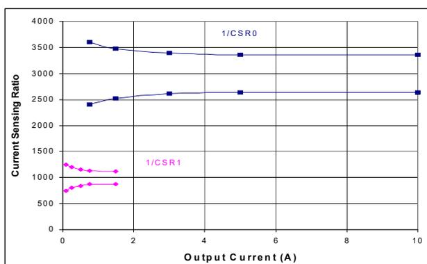
Figure 19. Current sensing ratio versus output current
