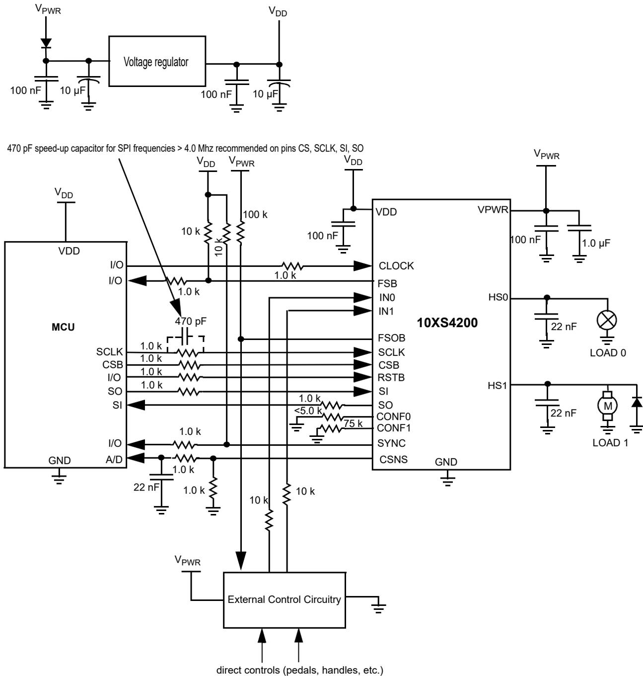
Figure 23. Typical application with two different load types
