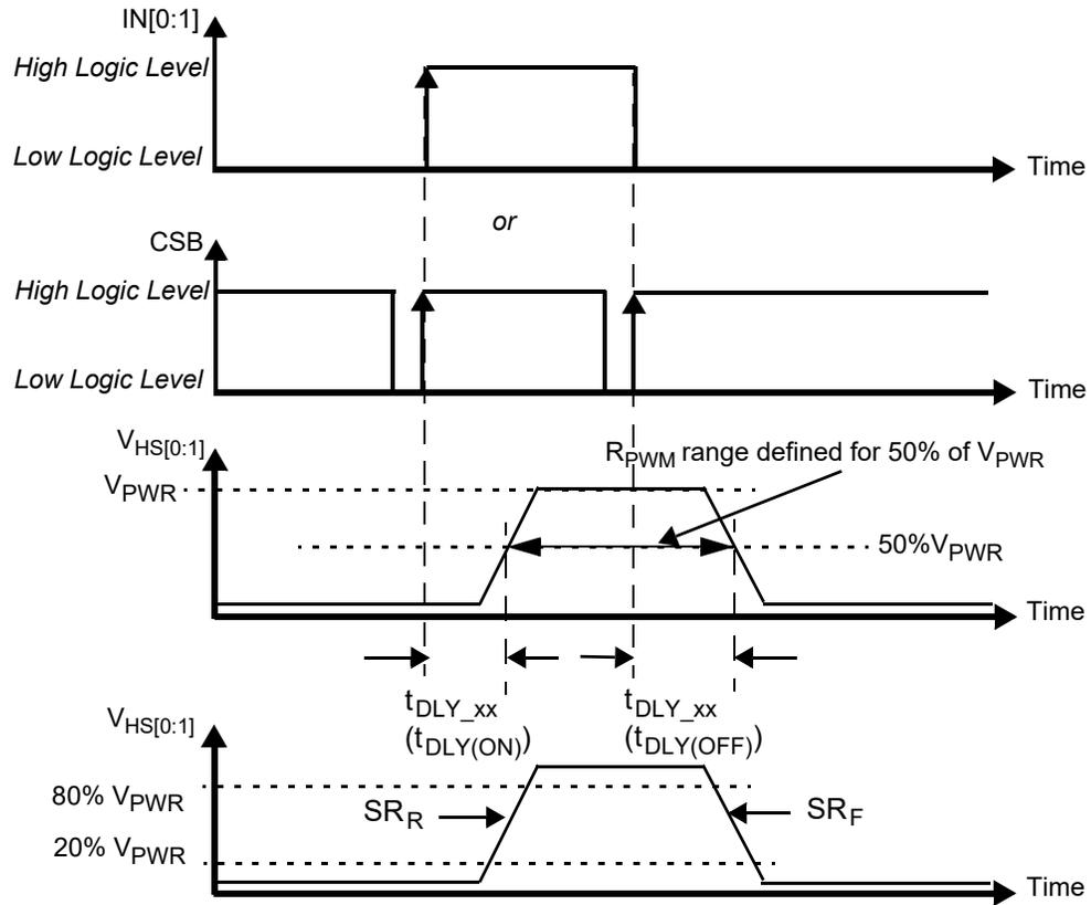
Figure 4. Output voltage slew rate and delay
