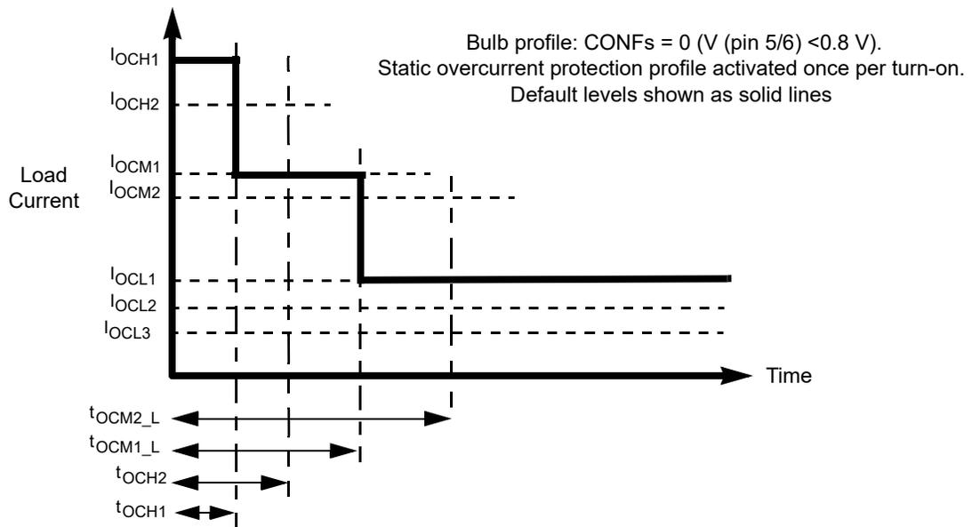
Figure 5. Overcurrent protection profile for bulb applications
