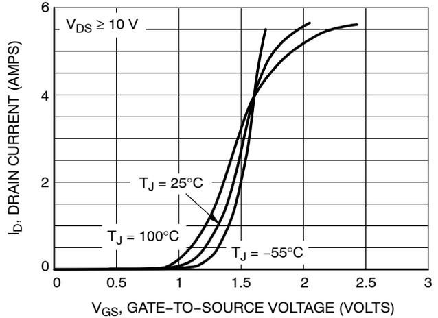
**Figure 2. Transfer Characteristics**
