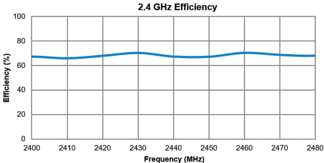
2.4 GHz embedded antenna specifications
