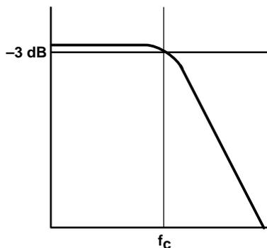
$$f_{c(\text{lowpass})} = \frac{1}{2\pi R_F C_F} \quad (7)$$
