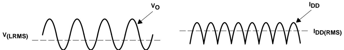
**Figure 25. Voltage and Current Waveforms for BTL Amplifiers**
