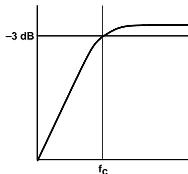
$$f_{c(\text{highpass})} = \frac{1}{2\pi R_I C_I} \quad (8)$$
